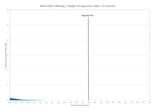
Below is same straight-through lanes as above but scaled to fit the entire y-axis. Like the turning lanes, the straight-through lanes show a curve which ends at the stopping time. Some vehicles decelerate on route to the intersection because of hazards, unexpected lane changes, etc:
