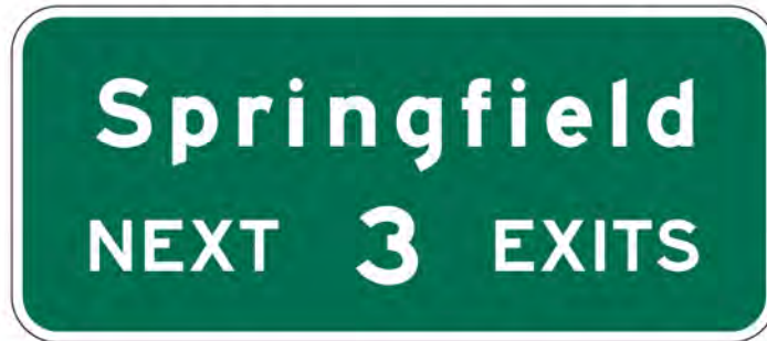
Figure 2E-33. NEXT EXITS Sign
