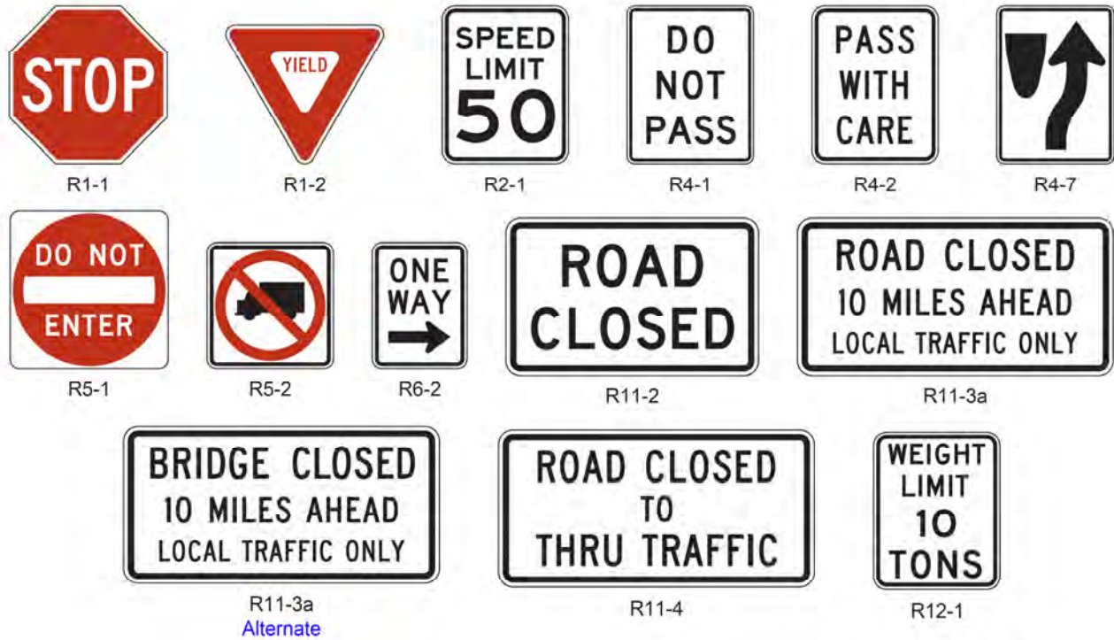
Figure 5B-1. Regulatory Signs on Low-Volume Roads
