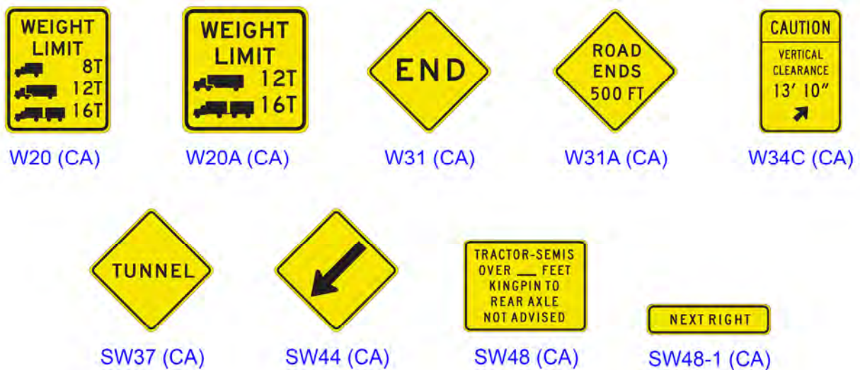
Figure 2C-5 (CA). Miscellaneous Warning Signs
