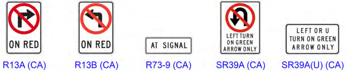
Figure 2B-27 (CA). Traffic Signal Signs and Plaques
