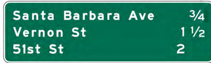
Figure 2E-31. Interchange Sequence Sign
