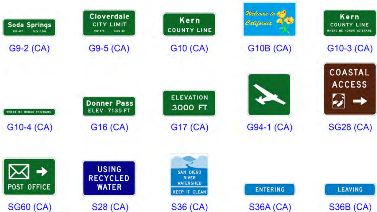
Figure 2H-1 (CA). General Information and Miscellaneous Information Signs
