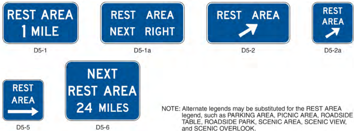
Figure 2I-5. Rest Area and Other Roadside Area Signs
