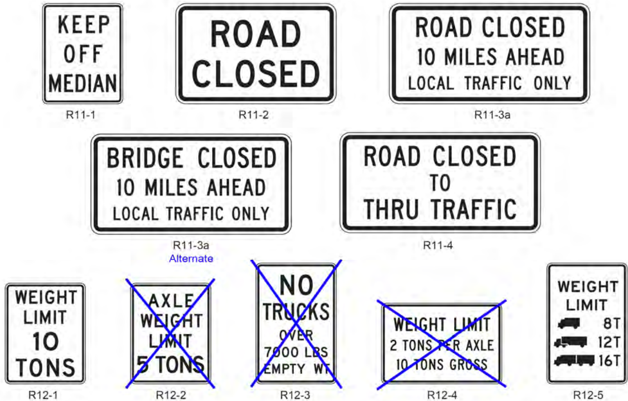
Figure 2B-29. Road Closed and Weight Limit Signs
