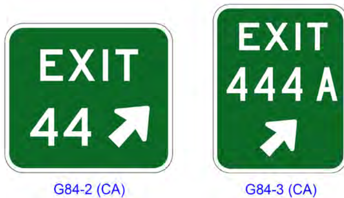
Figure 2E-28 (CA). Exit Gore Signs
