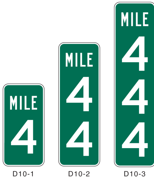
Figure 2H-2. Reference Location Signs
