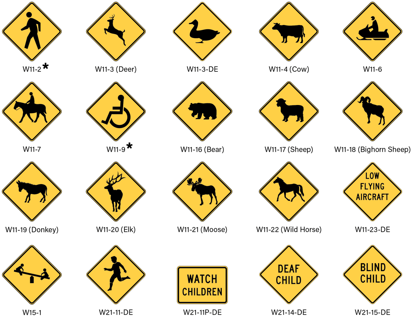
Figure 2C-11. Non-Vehicular Warning Signs (Delaware Revision)
