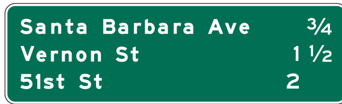
Figure 2E-31. Interchange Sequence Sign
