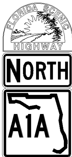
Figure 2.34-2. Co-Location on Route Confirmation Marker
