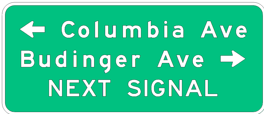
Figure 2.37-6. Advance Street Name Sign Using Different Names
