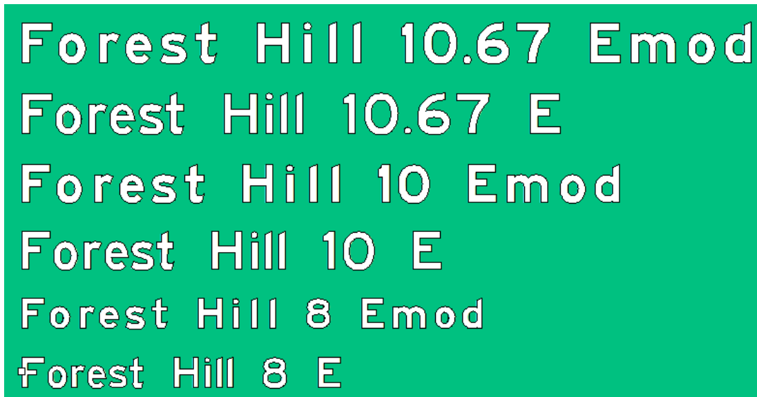
Figure 2.37-5. Standard Font Sizes for Advance Street Name Sign Legends
