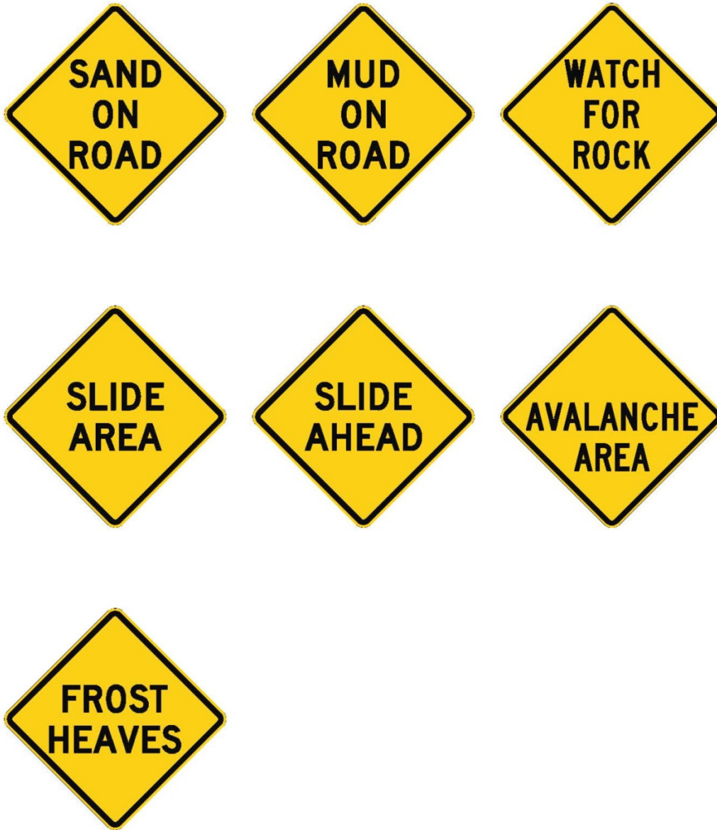
Figure 2C-3 Example Roadway Condition Signs
