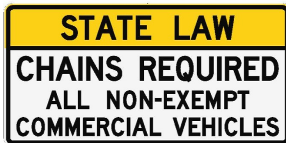
Figure 2B-10 Chains Required Sign
