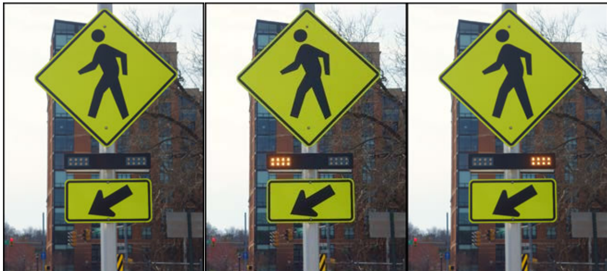
Figure 4L-1 Rectangular Rapid Flashing Beacon
