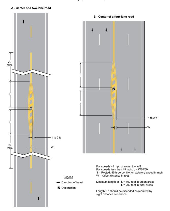
Figure 3B-15. Examples of Applications of Markings for Obstructions in the Roadway (Sheet 2 of 2)
