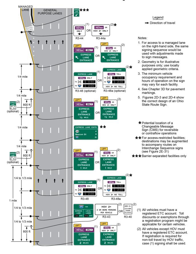
Figure 2G-22. Example of Signing for the Entrance to an Access-Restricted Priced Managed Lane Where a General-Purpose Lane Becomes the Managed Lane
