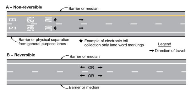
Figure 3D-2. Markings for Buffer-Separated Preferential Lanes (Sheet 1 of 2)
