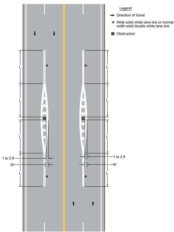
For speeds of 45 mph or more: L = WS For speeds of less than 45 mph: L = WS<sup>2</sup>/60 S = Posted, 85th-percentile, or statutory speed in mph W = Offset distance in feet Minimum length of: L = 100 feet in urban areas L = 200 feet in rural areas
