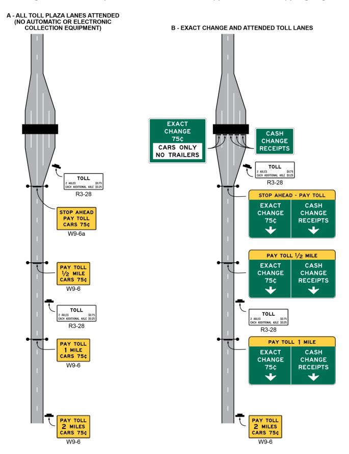
Figure 2F-11. Examples of Guide Signs for a Mainline Toll Plaza on a Diverging Alignment from Open-Road ETC Lanes
