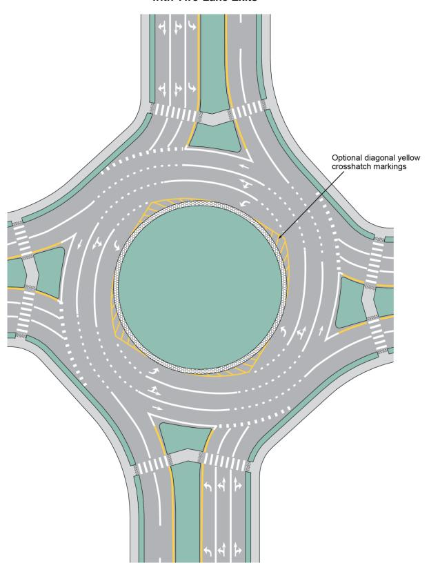
Figure 3C-13. Example of Markings for Two Linked Roundabouts
