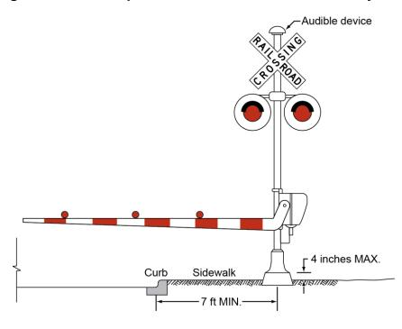
Figure 8C-6. Example of a Separate Pedestrian Gate
