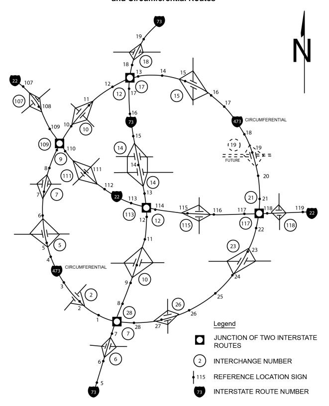
Figure 2E-20. Example of Interchange Numbering for Mainline, Loop, and Spur Routes
