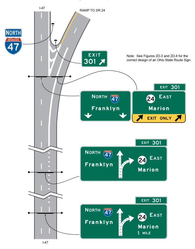
Figure 2E-9. Diagrammatic Guide Signs for a Two-Lane Exit to the Right with an Optional Lane (Through Lanes Curve to the Left)
