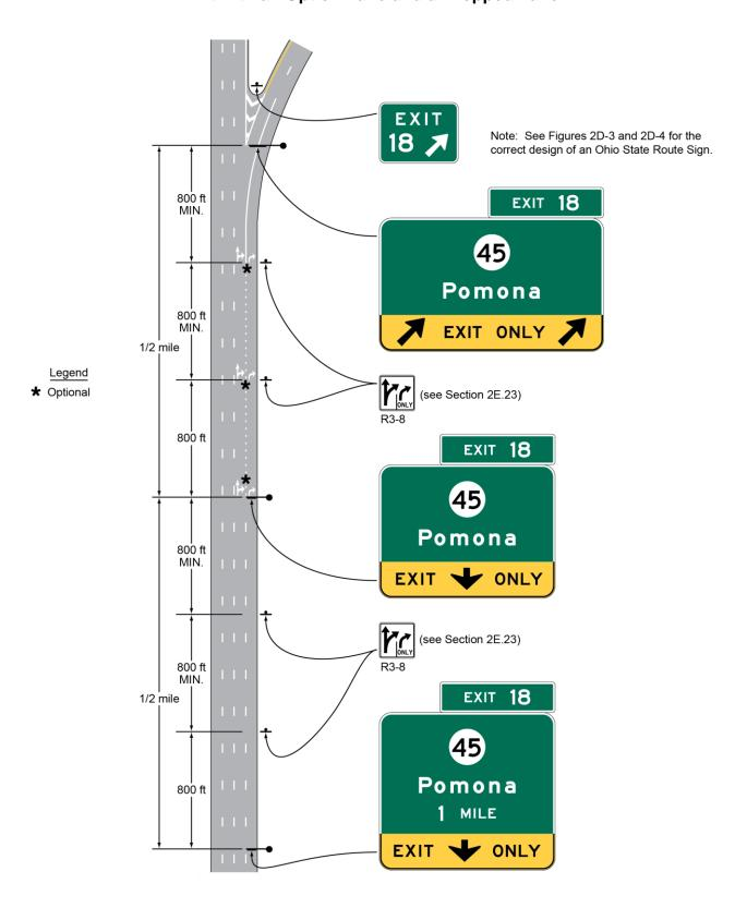
Figure 2E-12. Example of Signing for a Two-Lane Intermediate or Minor Interchange Exit with Option and Auxiliary Lanes
