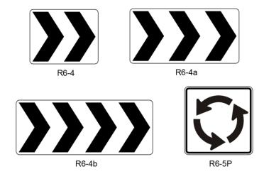
Figure 2B.21. Example of Regulatory and Warning Signs for a Mini-Roundabout
