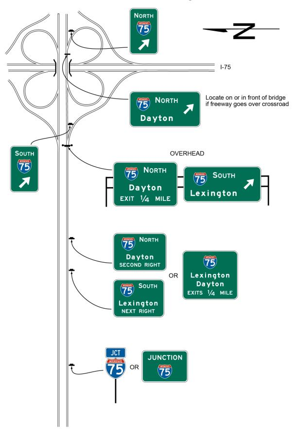
Figure 2D-16. Example of Crossroad Signing for an Entrance Ramp with a Nearby Frontage Road
