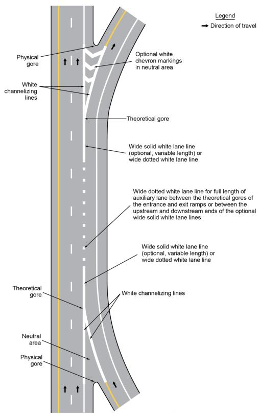
Figure 3B-11. Examples of Applications of Conventional Road Lane-Drop Markings (Sheet 1 of 2)
