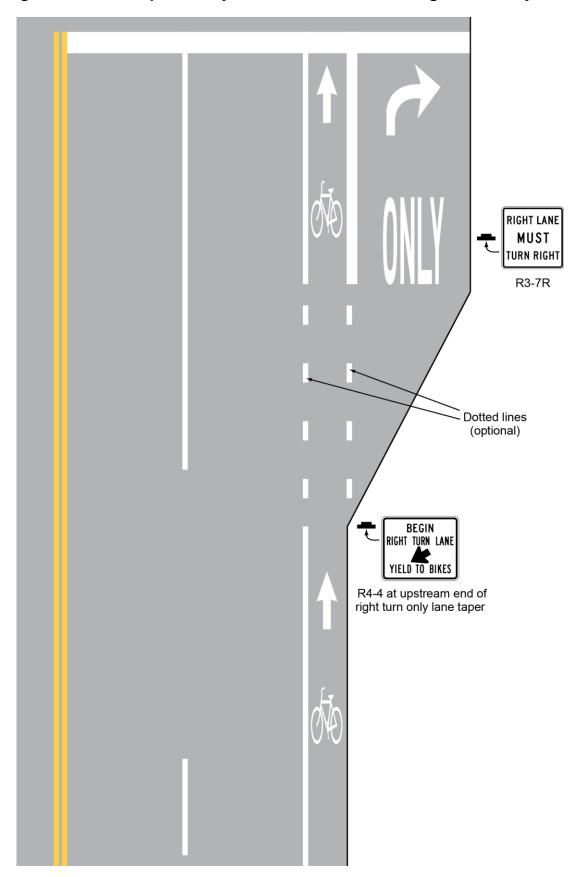
Figure 9C-5. Example of Bicycle Lane Treatment at Parking Lane into a Right Turn Only Lane
