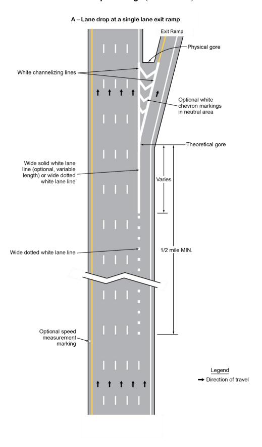
Figure 3B-10. Example of Applications of Freeway and Expressway Lane Drop Markings (Sheet 2 of 5)
