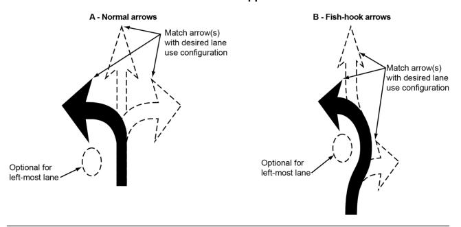
Figure 3C-3. Example of Markings for a One-Lane Roundabout
