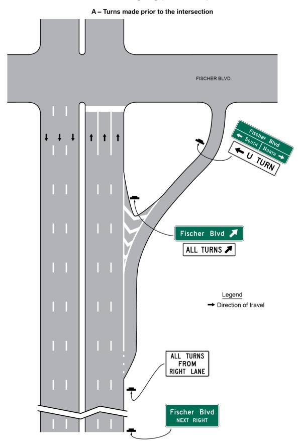
Figure 2B-9. Examples of Applications of Jughandle Regulatory and Guide Signing (Sheet 2 of 3)
