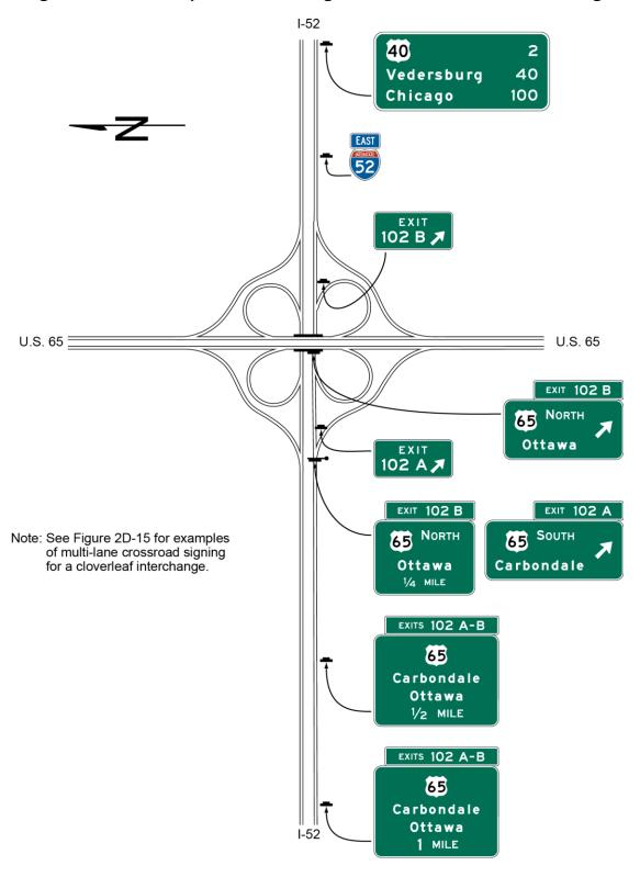
Figure 2E-36. Examples of Guide Signs for Full Cloverleaf Interchange with Collector-Distributor Roadways
