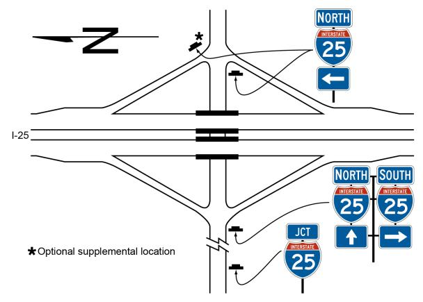
Figure 2D-13. Examples of Multi-Lane Crossroad Signing for a Diamond Interchange
