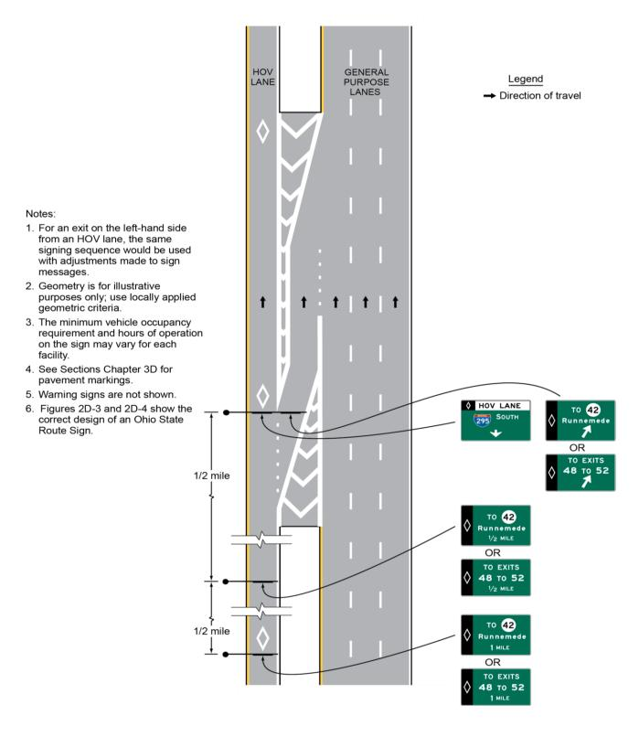
Figure 2G-13. Example of Signing for a Direct Entrance Ramp to an HOV Lane from a Park – Ride Facility and a Local Street
