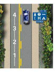
Drivers need to change following distance when speed or road conditions change. Hand response time is close to a half second. Foot response time is normally three-quarters of a second. This does not take into account any delay in perception time as a result of the driver being tired, on medication, distracted, etc. Road conditions, speed, driver alertness, and even following vehicles of different weights all change the ability to stop.
