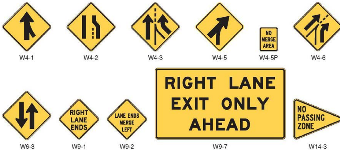
Figure 2C-8. Merging and Passing Signs and Plaques
