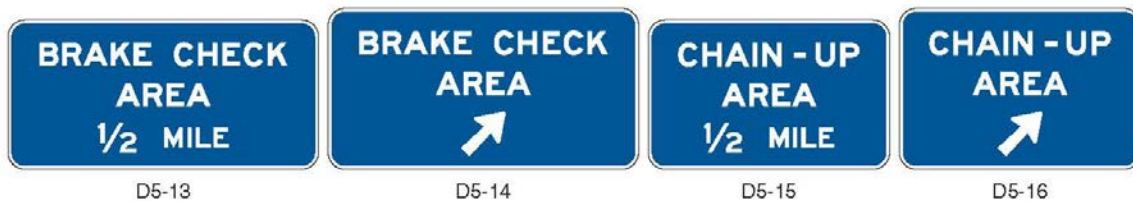
Figure 2I-6. Brake Check Area and Chain-Up Area Signs
