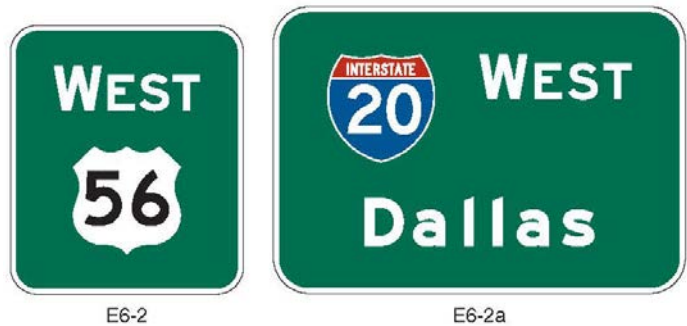
Figure 2E-2. Pull-Through Signs
