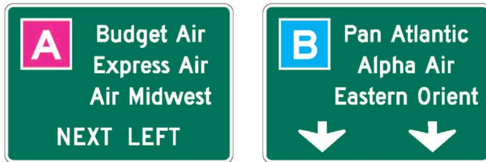
Figure 2D-1. Examples of Color-Coded Destination Guide Signs
