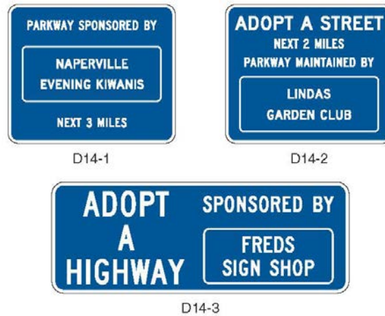
Figure 2H-5. Examples of Acknowledgment Sign Designs
