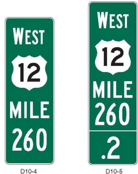
Figure 2H-4. Enhanced Reference Location Signs
