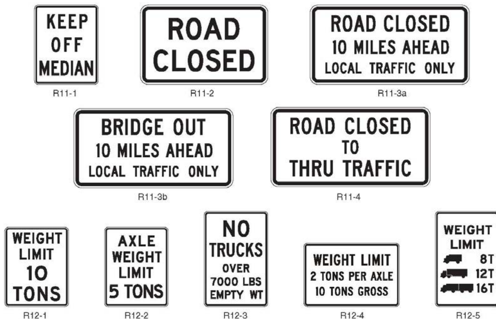
Figure 2B-29. Road Closed and Weight Limit Signs
