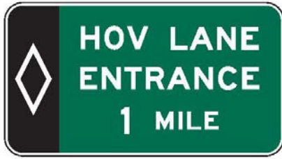
Figure 2G-5. Example of an Overhead Advance Guide Sign for a Preferential Lane Entrance
