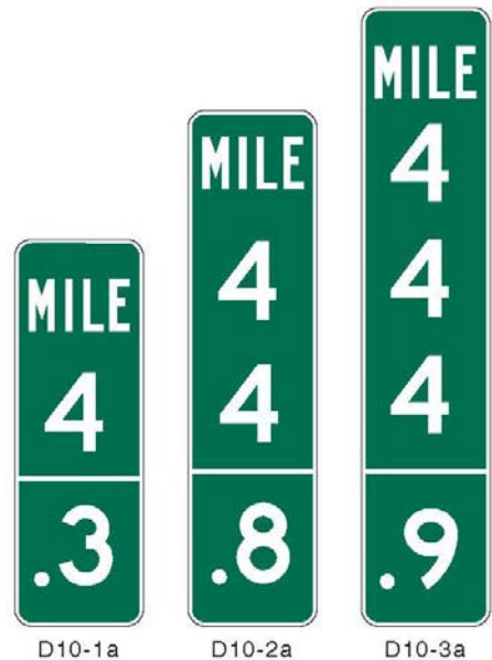
Figure 2H-3. Intermediate Reference Location Signs
