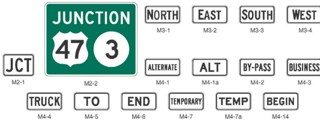
Figure 2D-4. Route Sign Auxiliaries
