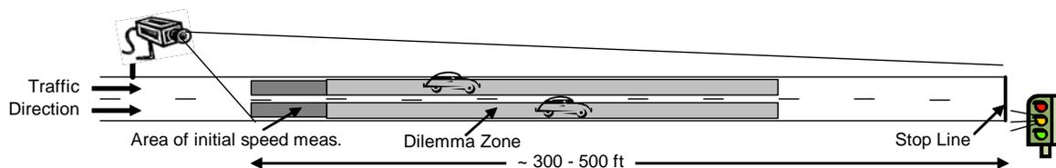
**FIGURE 2 Field setup for video recording of driver behavior data.**
