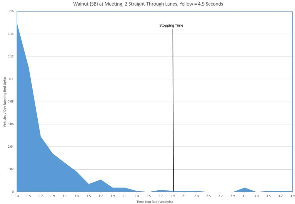
Minor changes in the yellow light duration radically affect the red light running rate. I also have [a plot of counts vs. time](#) for every red light camera intersection in Cary. Every time Cary decreases or increases the yellow, the counts radically spike or dip to permanent new levels. Even a 0.1 second decrease in the yellow increases the violation rate by 50%.
