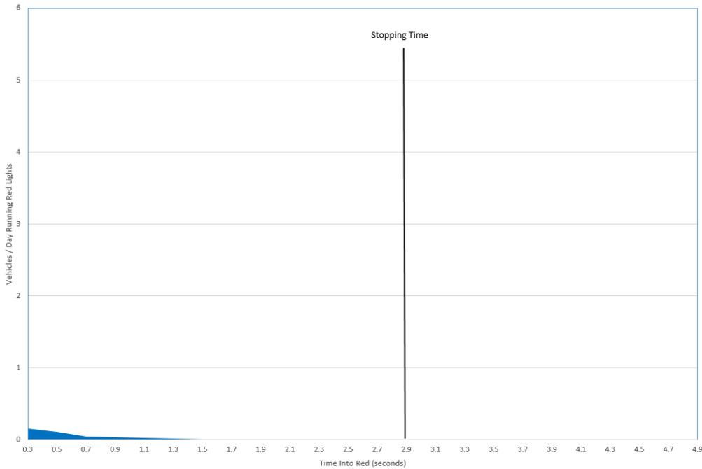
Below is same straight-through lanes as above but scaled to fit the entire y-axis. Like the turning lanes, the straight-through lanes show a curve which ends at the stopping time. Some vehicles decelerate on route to the intersection because of hazards, unexpected lane changes, etc:
