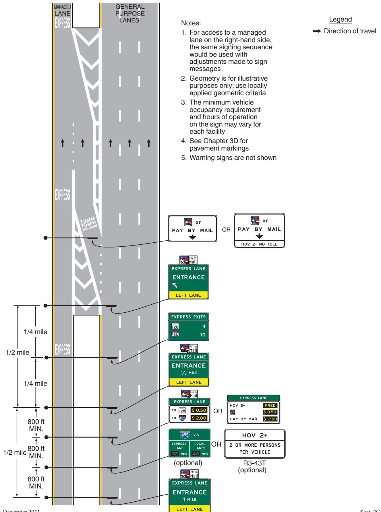
**Figure 2G-24T. Example of Signing for the Intermediate Entry to, Egress from, and End of Access-Restricted Priced Express Lanes**
