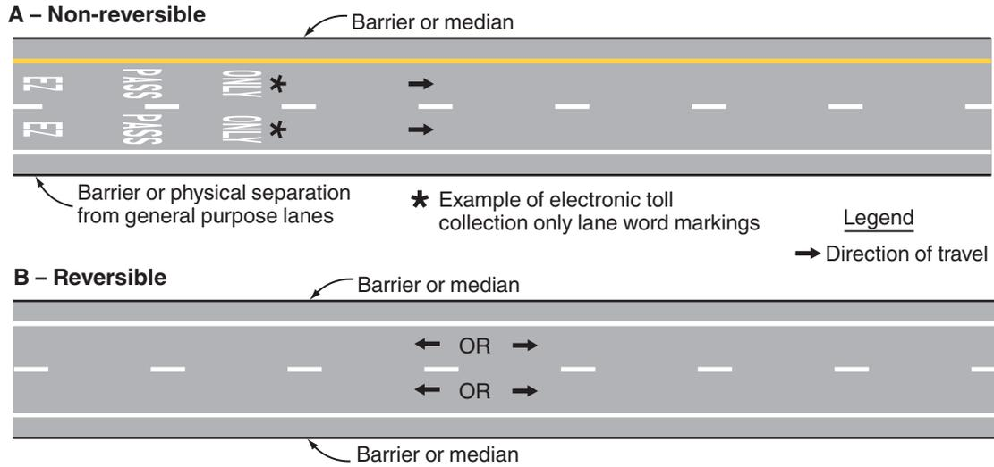
**Figure 3D-2. Markings for Buffer-Separated Preferential Lanes (Sheet 1 of 2)**
