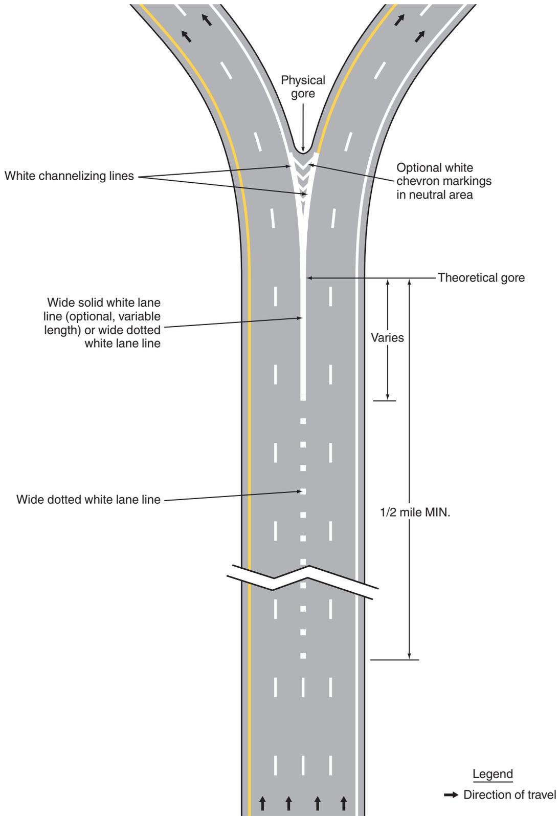
**Figure 3B-10. Examples of Applications of Freeway and Expressway Lane-Drop Markings (Sheet 5 of 5)**
