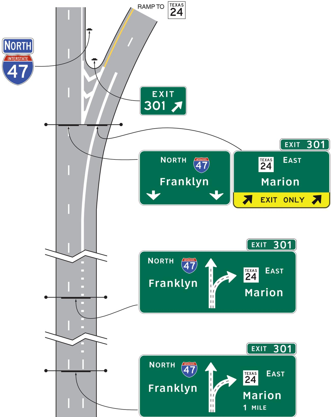
**Figure 2E-9. Diagrammatic Guide Signs for a Two-Lane Exit to the Right with an Option Lane (Through Lanes Curve to the Left)**
