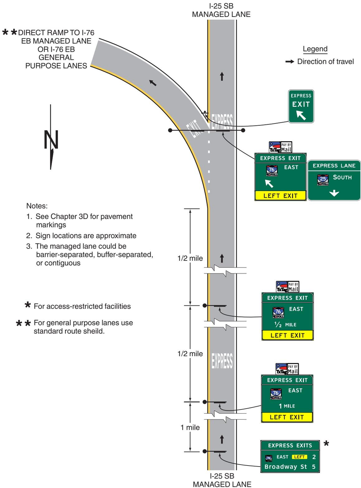
**Figure 2G-27TA. Examples of Guide Signs for a Direct Access Ramp to General Purpose Lanes**
