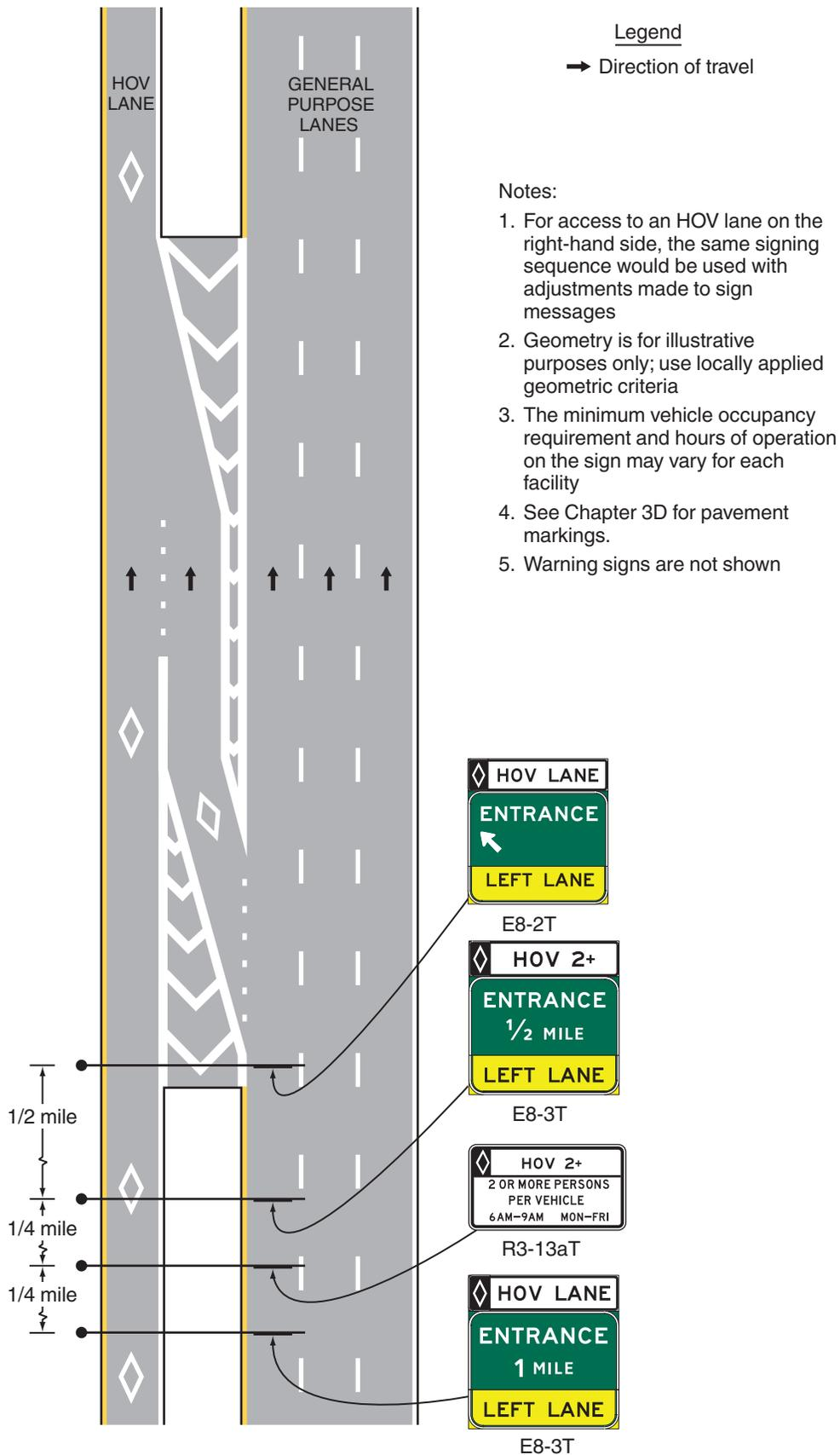
**Figure 2G-10. Example of Signing for the Intermediate Entry to, Egress from, and End of Access-Restricted HOV Lanes**
