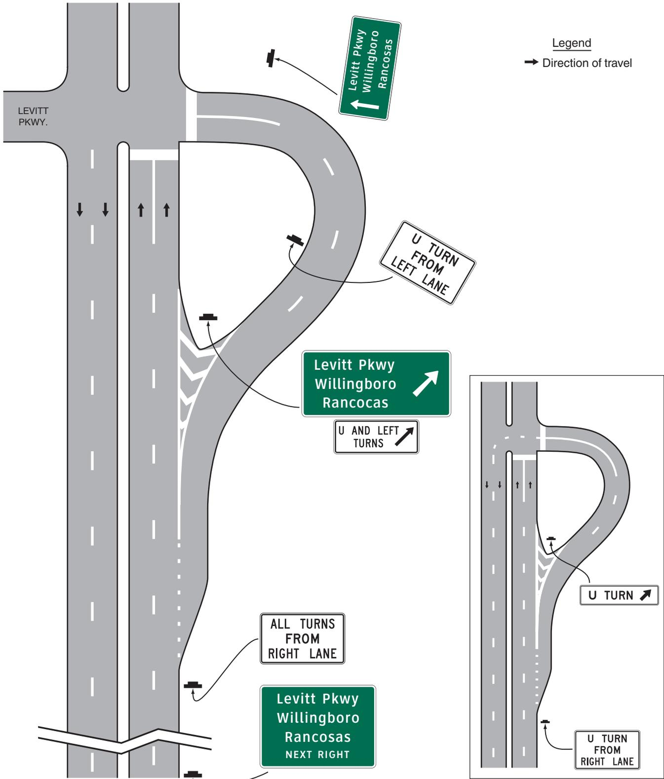
**Figure 2B-9. Examples of Applications of Jughandle Regulatory and Guide Signing**
