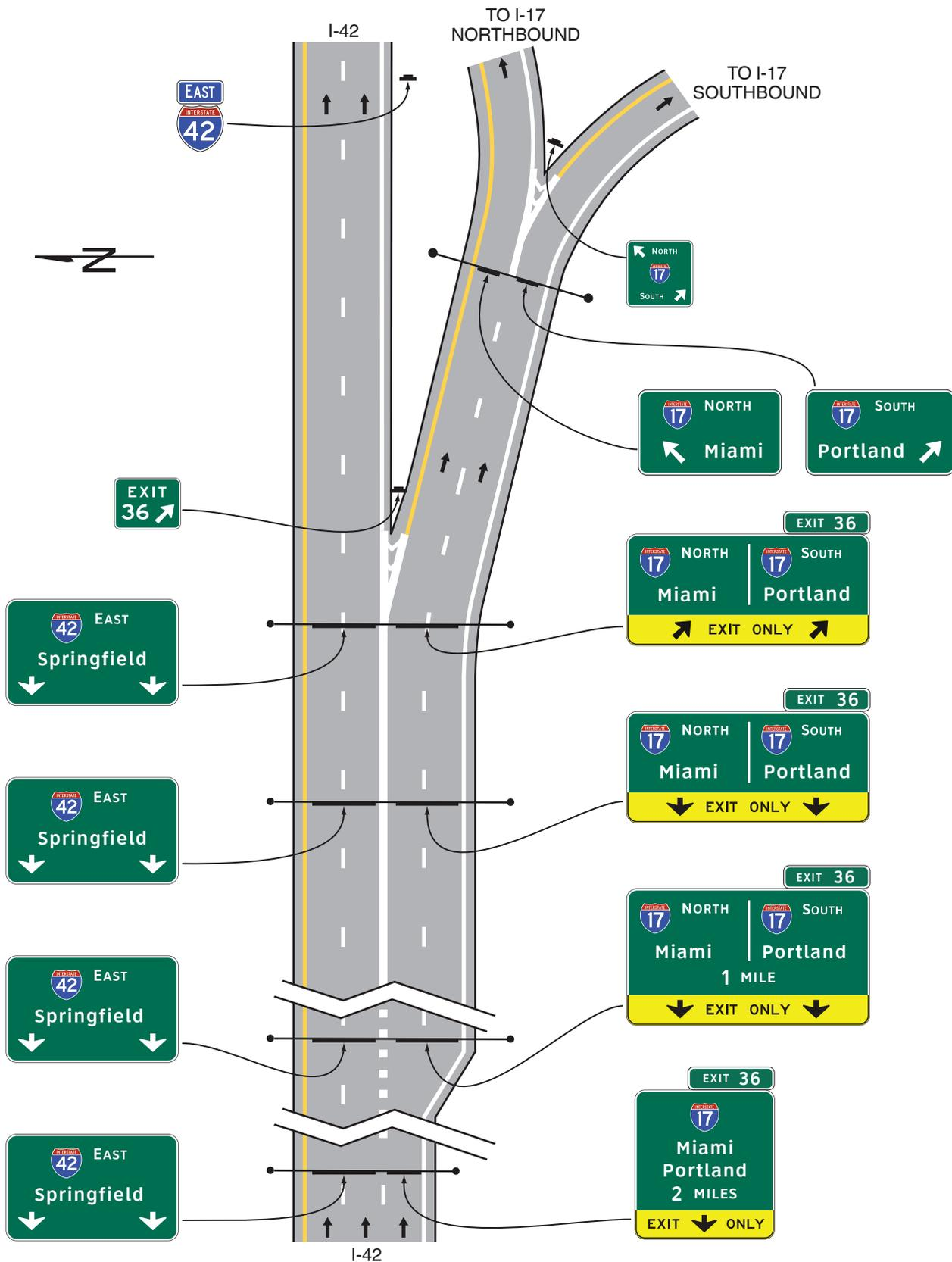
**Figure 2E-34. Examples of Guide Signs for a Freeway-to-Freeway Interchange**
