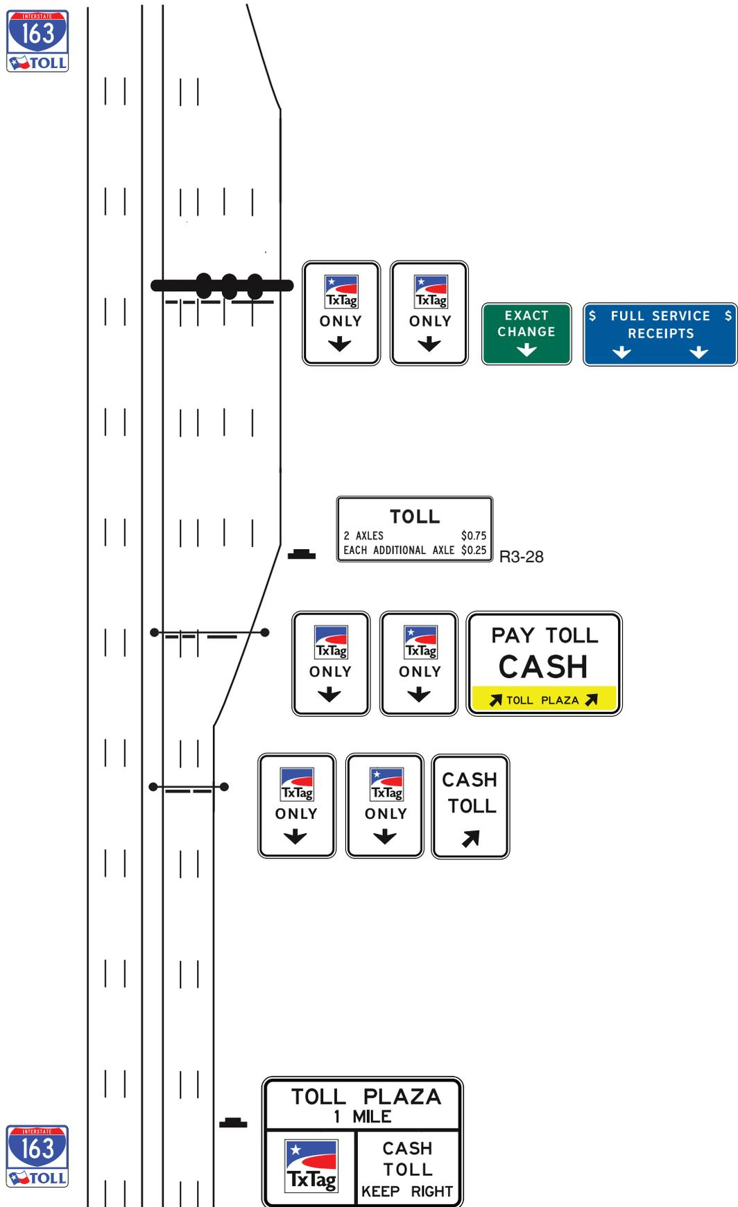
**Figure 2F-10TB. Examples of Guide Signs for a Mainlane Toll Plaza on a Diverging Alignment from Open-Road ETC Lanes with Video Billing**
