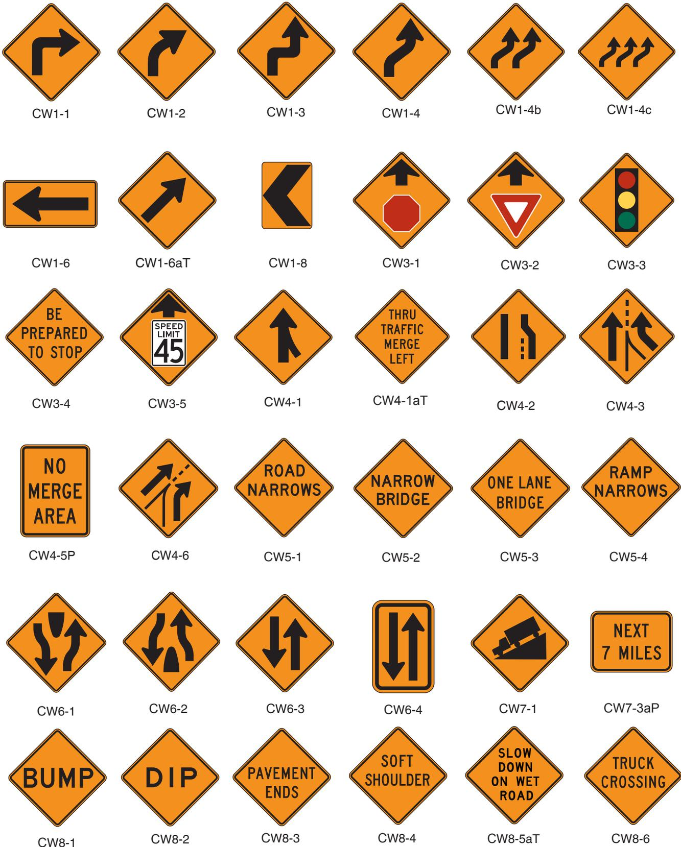
**Figure 6F-4. Warning Signs and Plaques in Temporary Traffic Control Zones**
