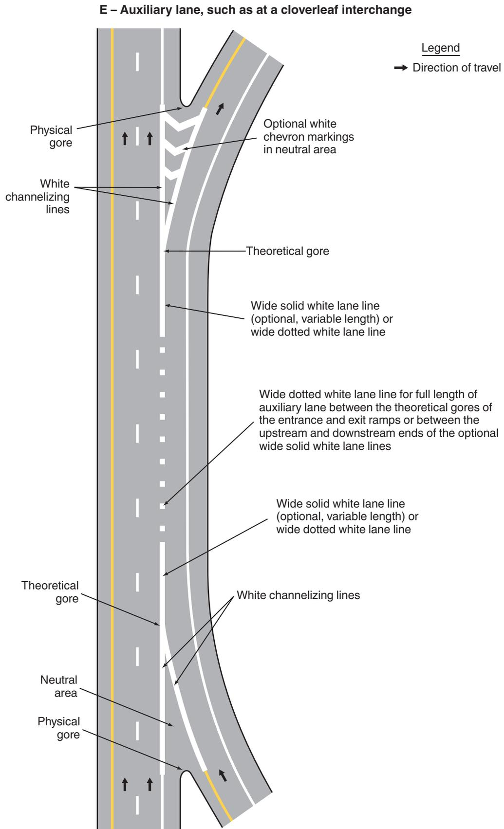
**Figure 3B-11. Examples of Applications of Conventional Road Lane-Drop Markings**
