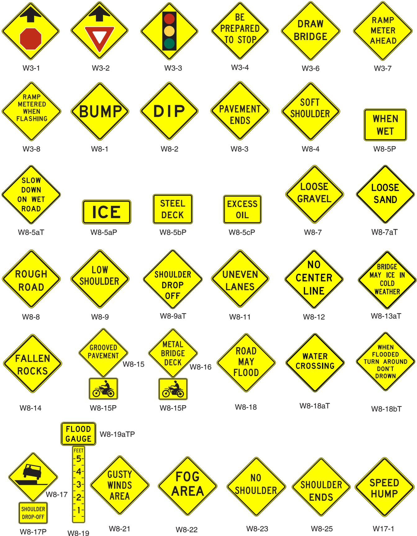
**Figure 2C-6. Roadway and Weather Condition and Advance Traffic Control Signs and Plaques (2 of 2)**
