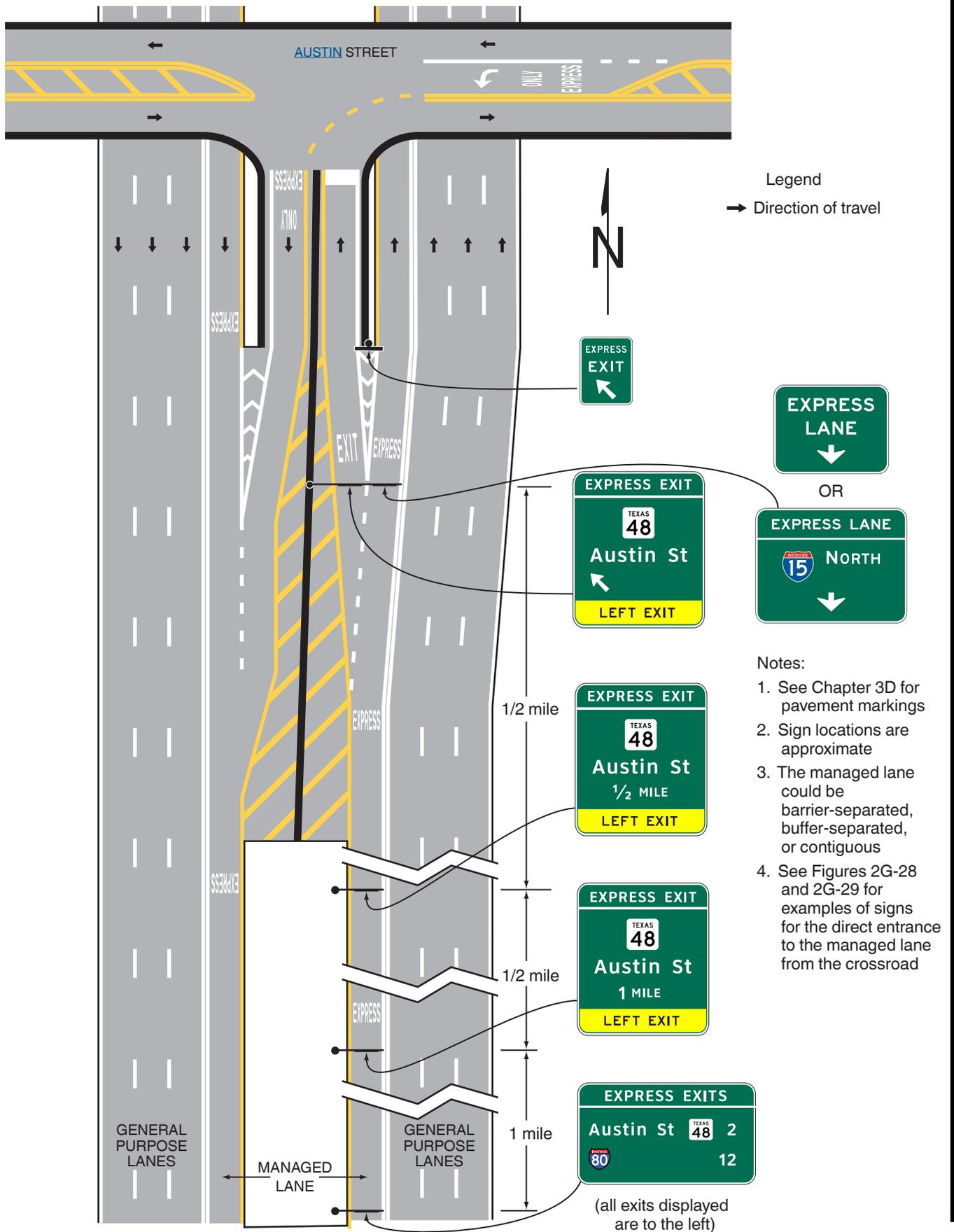
**Figure 2G-27. Examples of Guide Signs for a Direct Access Ramp to Managed Lane**
