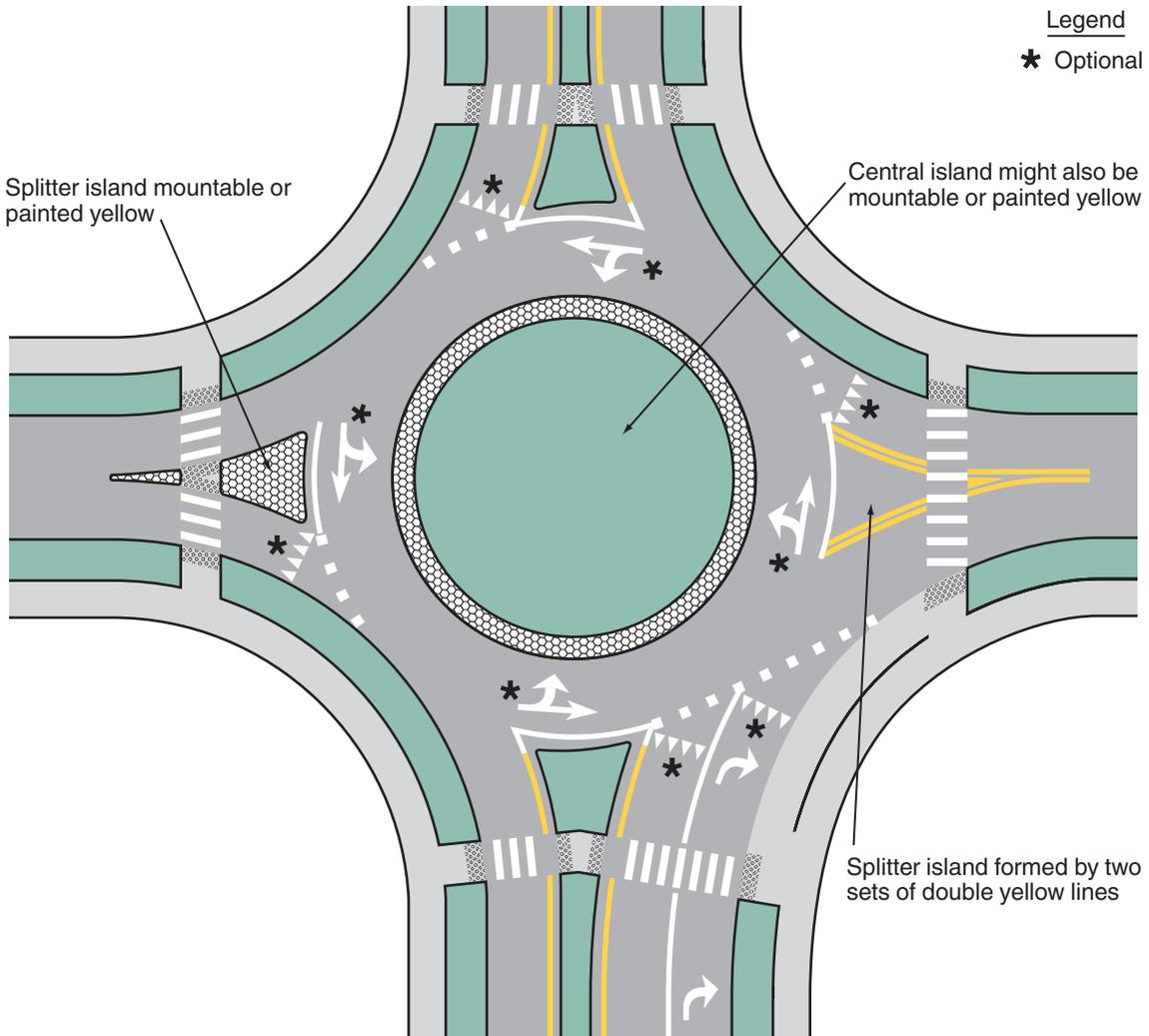
**Figure 3C-4. Example of Markings for a Two-Lane Roundabout with One- and Two-Lane Approaches (Sheet 1 of 2)**
