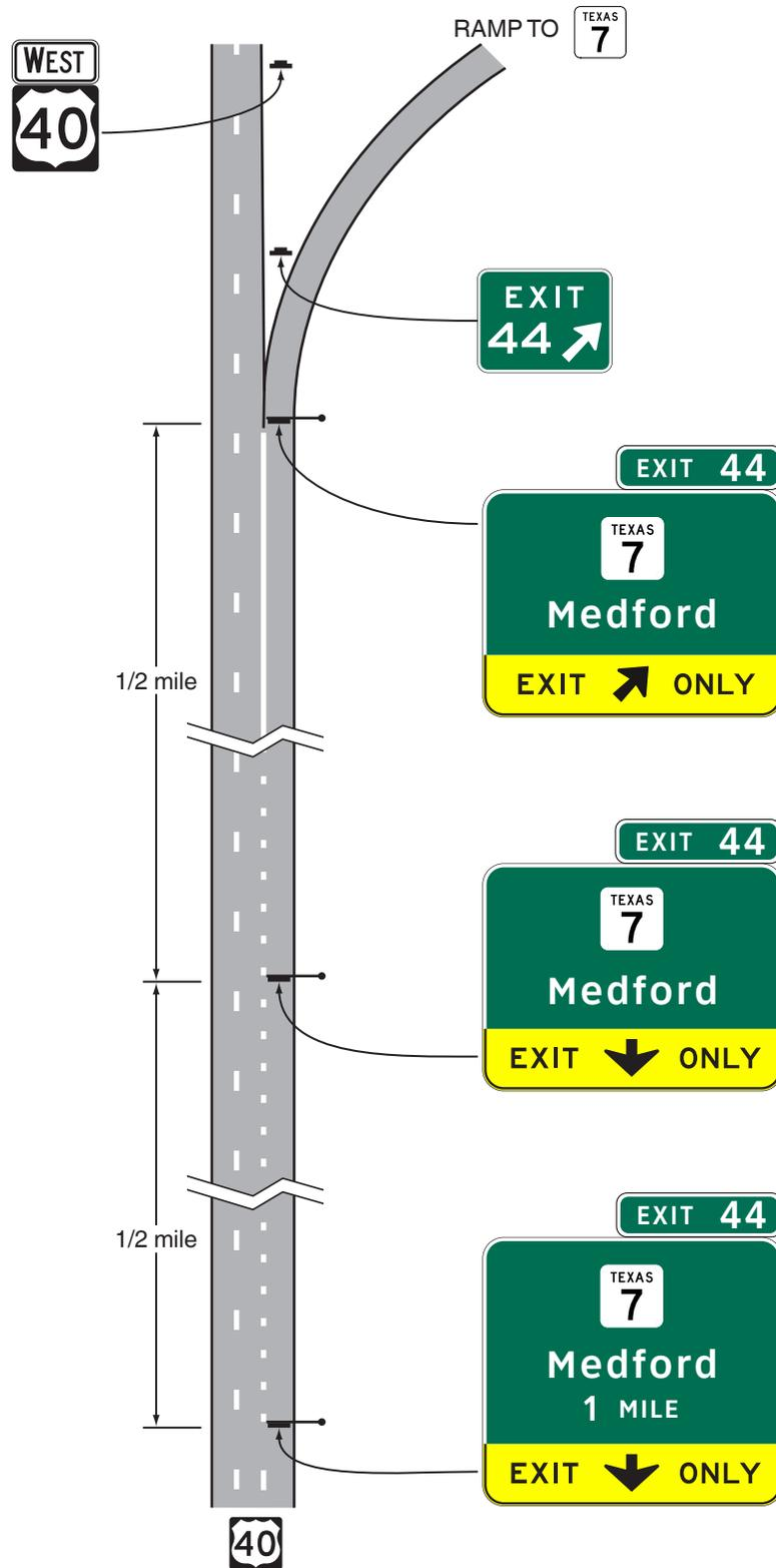
**Figure 2E-16TA. Guide Signs for a Single-Left Lane Exit**
