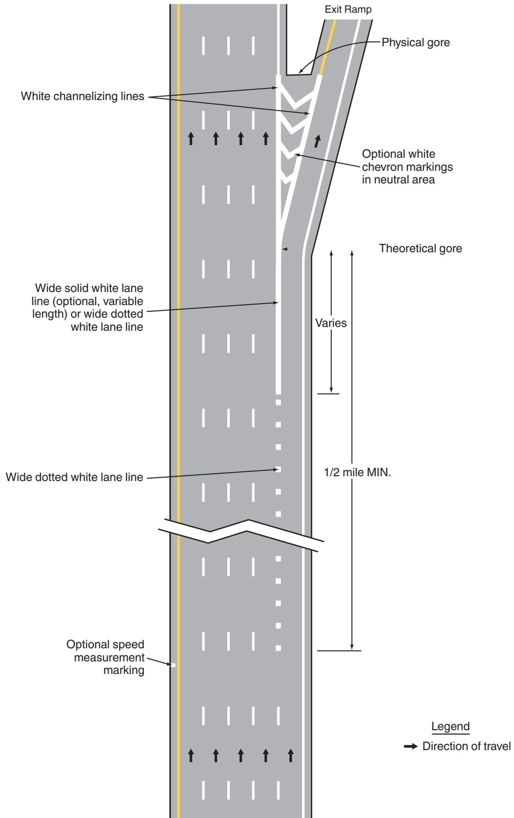
**Figure 3B-10. Examples of Applications of Freeway and Expressway Lane-Drop Markings (Sheet 3 of 5)**
