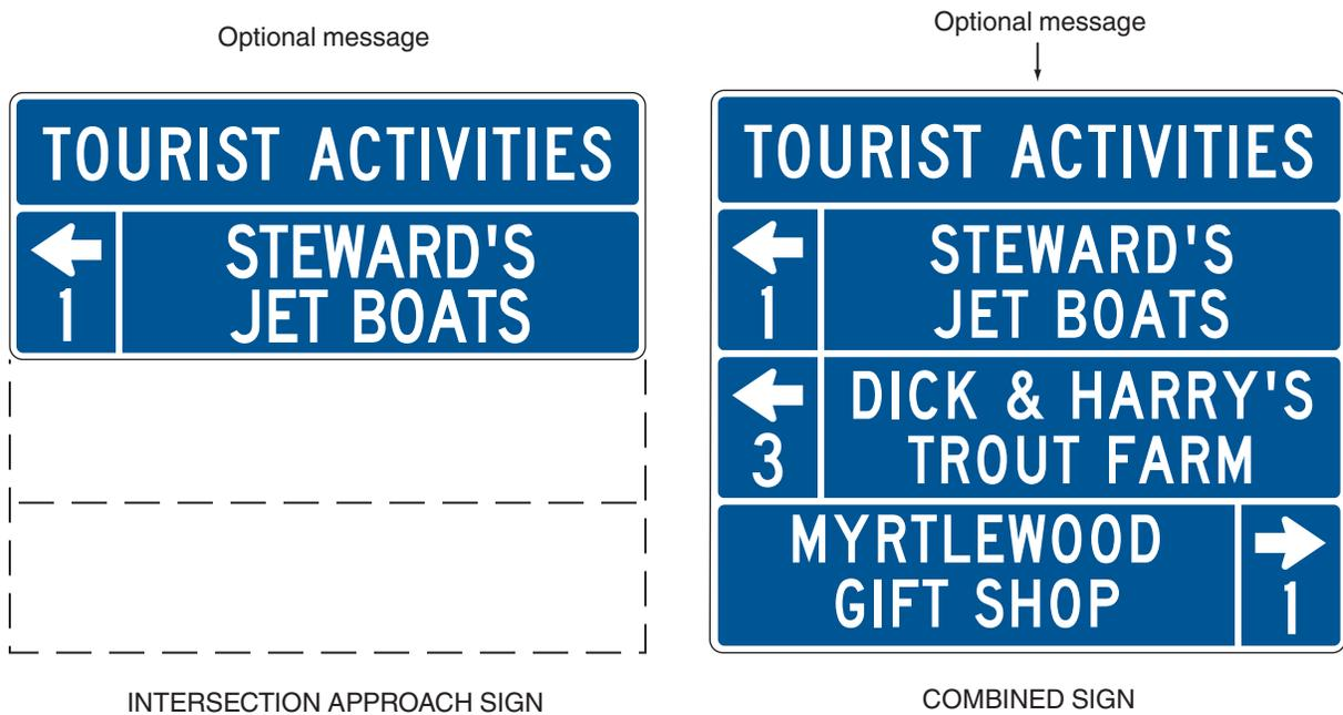
**Figure 2K-2. Examples of Intersection Approach Signs and Advance Signs for Tourist-Oriented Directional Signs**
