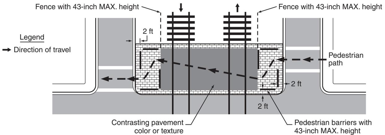
**Figure 8C-10. Examples of Pedestrian Barrier Installation at an Offset Non-Intersection Grade Crossing**
