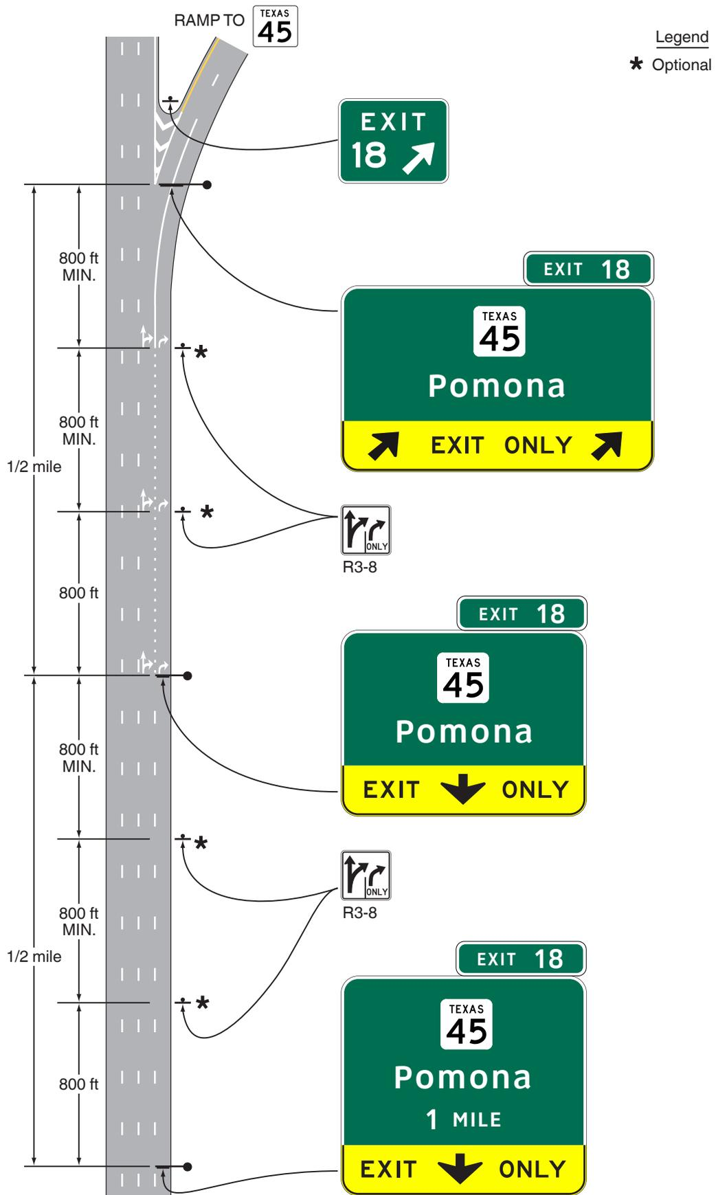
**Figure 2E-12. Example of Signing for a Two-Lane Intermediate or Minor Interchange Exit with Option and Auxiliary Lanes**
