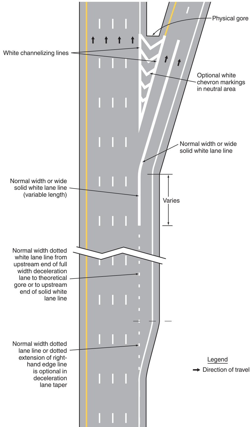
**Figure 3B-9. Examples of Dotted Line and Channelizing Line Applications for Entrance Ramp Markings (Sheet 1 of 2)**
