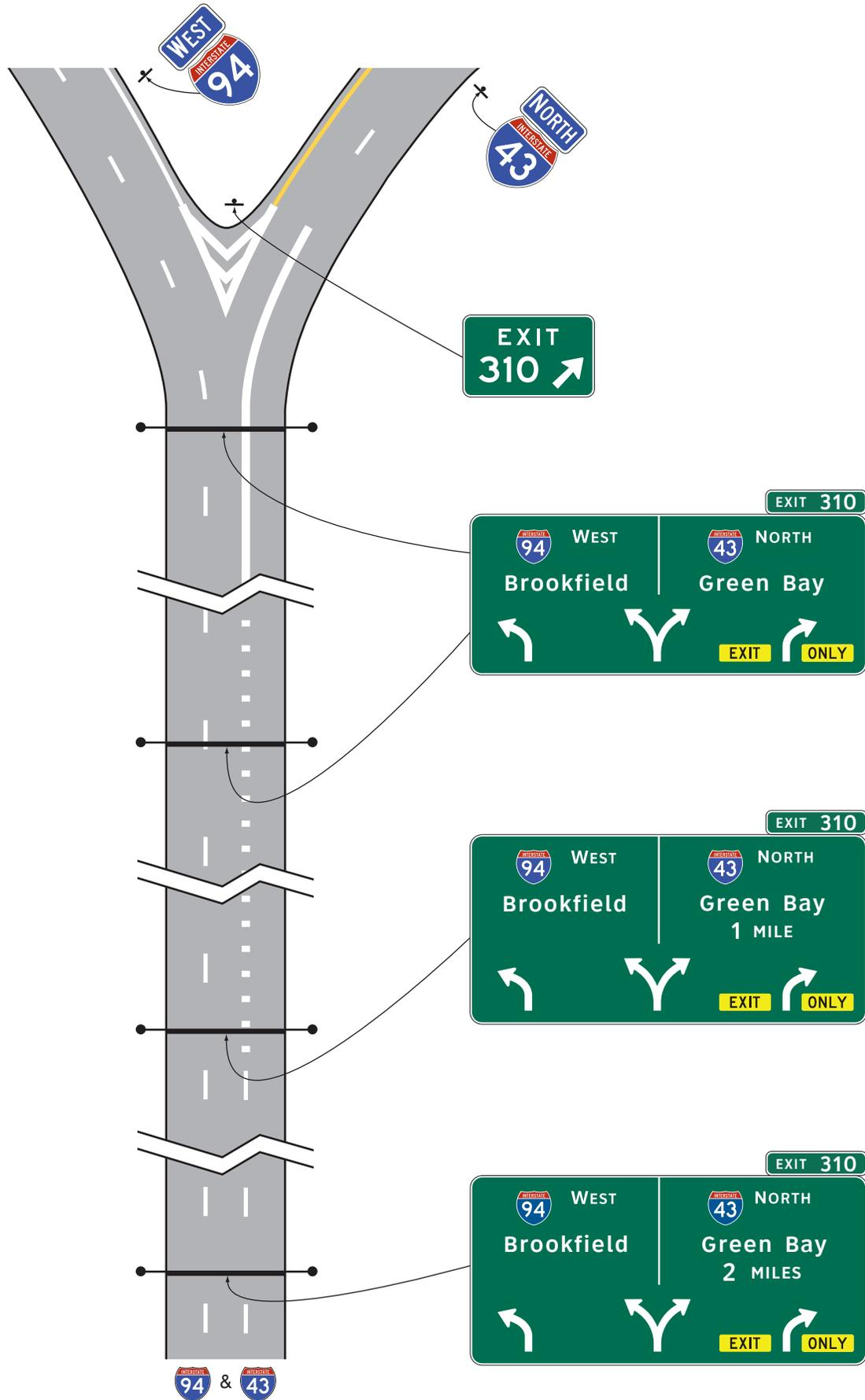
**Figure 2E-7. Diagrammatic Guide Sign for a Multi-Lane Exit with an Option Lane**
