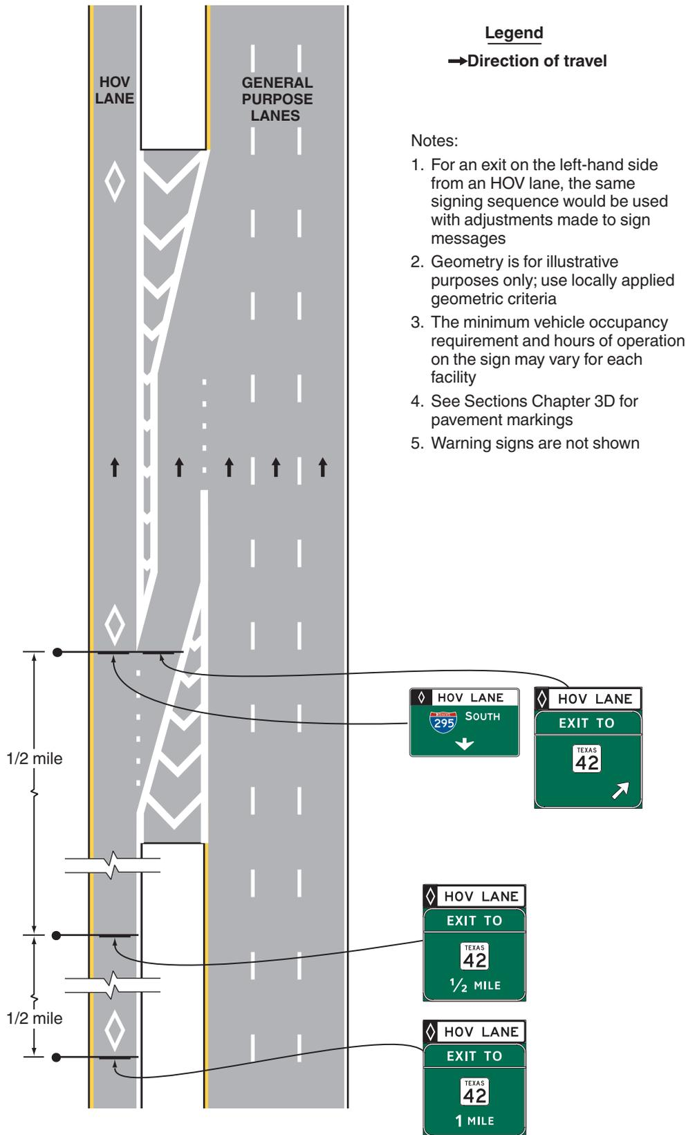
**Figure 2G-13. Example of Signing for a Direct Entrance Ramp to an HOV Lane from a Park-and-Ride Facility and a Local Street**
