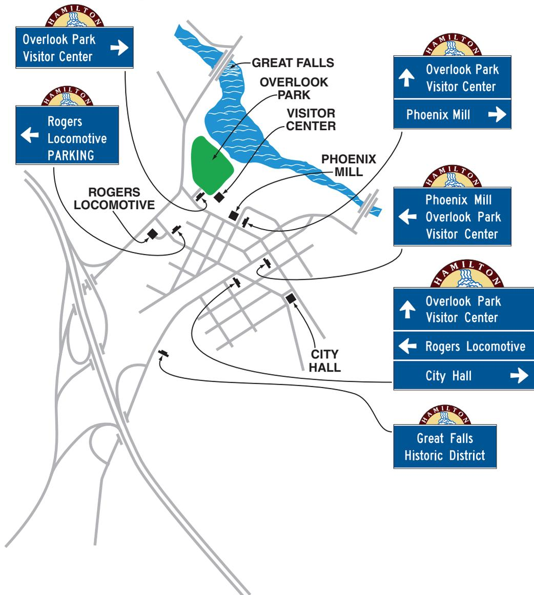
**Figure 2D-20. Example of a Color-Coded Community Wayfinding Guide Sign System**
