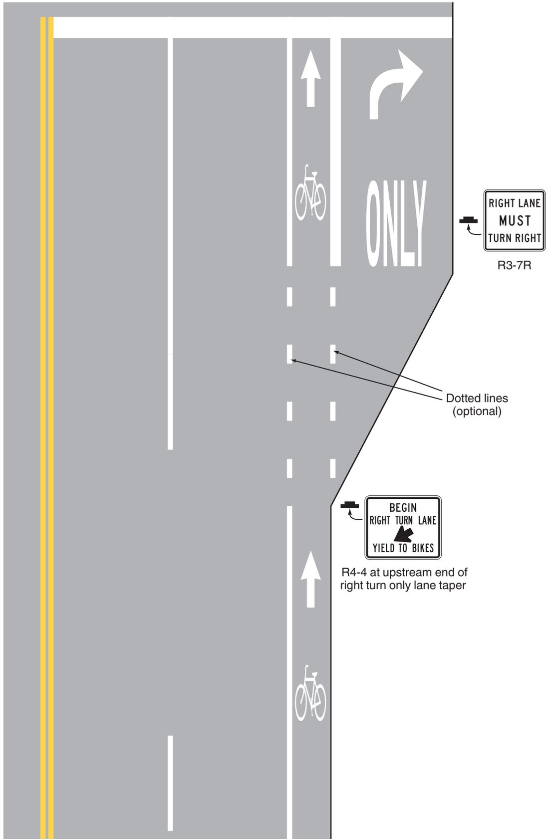
**Figure 9C-5. Example of Bicycle Lane Treatment at Parking Lane into a Right Turn Only Lane**
