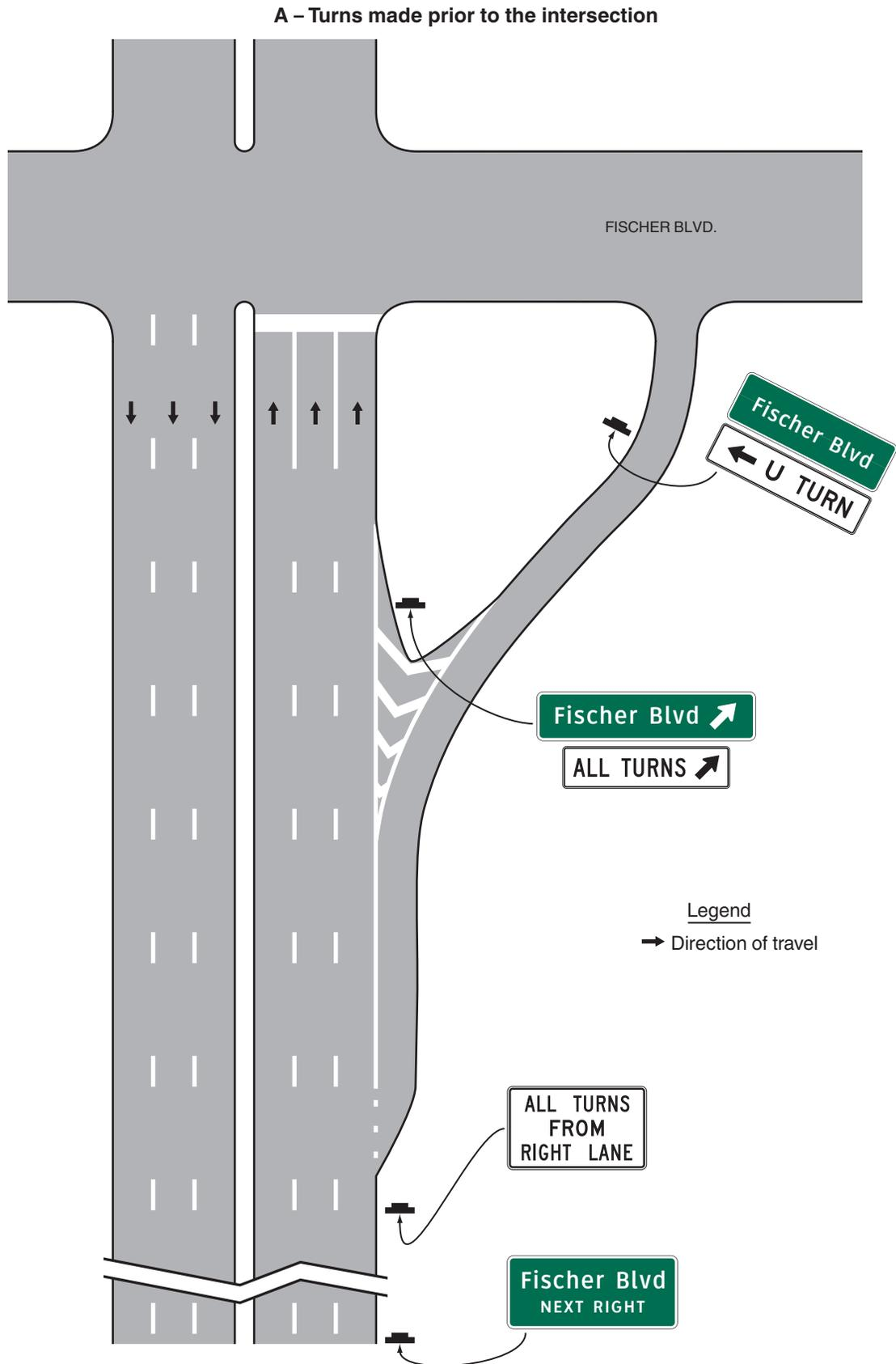
**Figure 2B-9. Examples of Applications of Jughandle Regulatory and Guide Signing**
