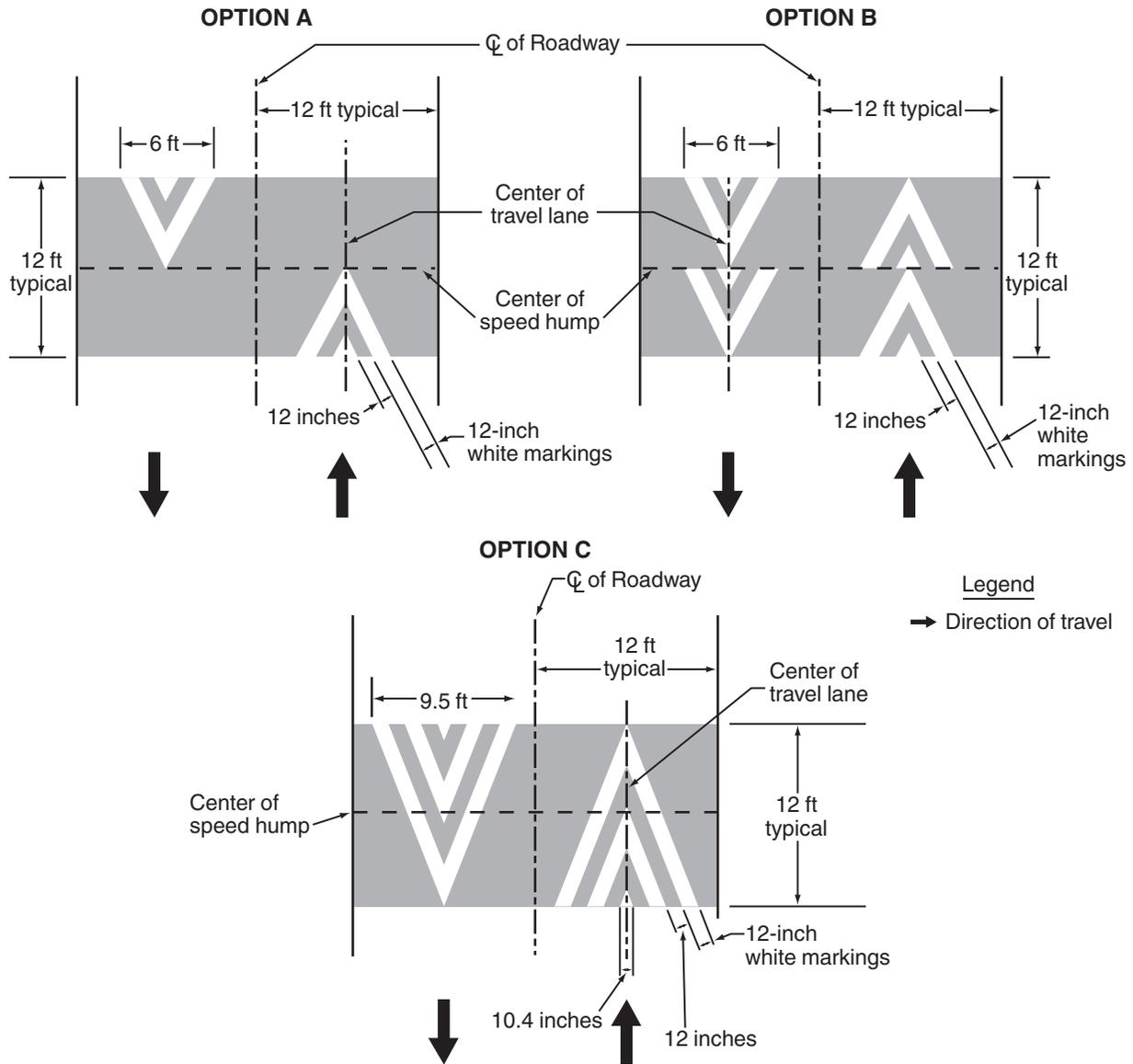
**Figure 3B-31. Advance Warning Markings for Speed Humps**
