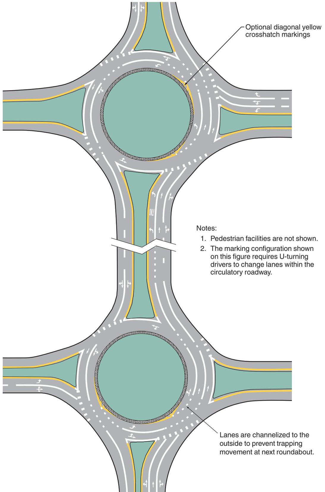
**Figure 3C-14. Example of Markings for a Diamond Interchange with Two Circular-Shaped Roundabout Ramp Terminals**
