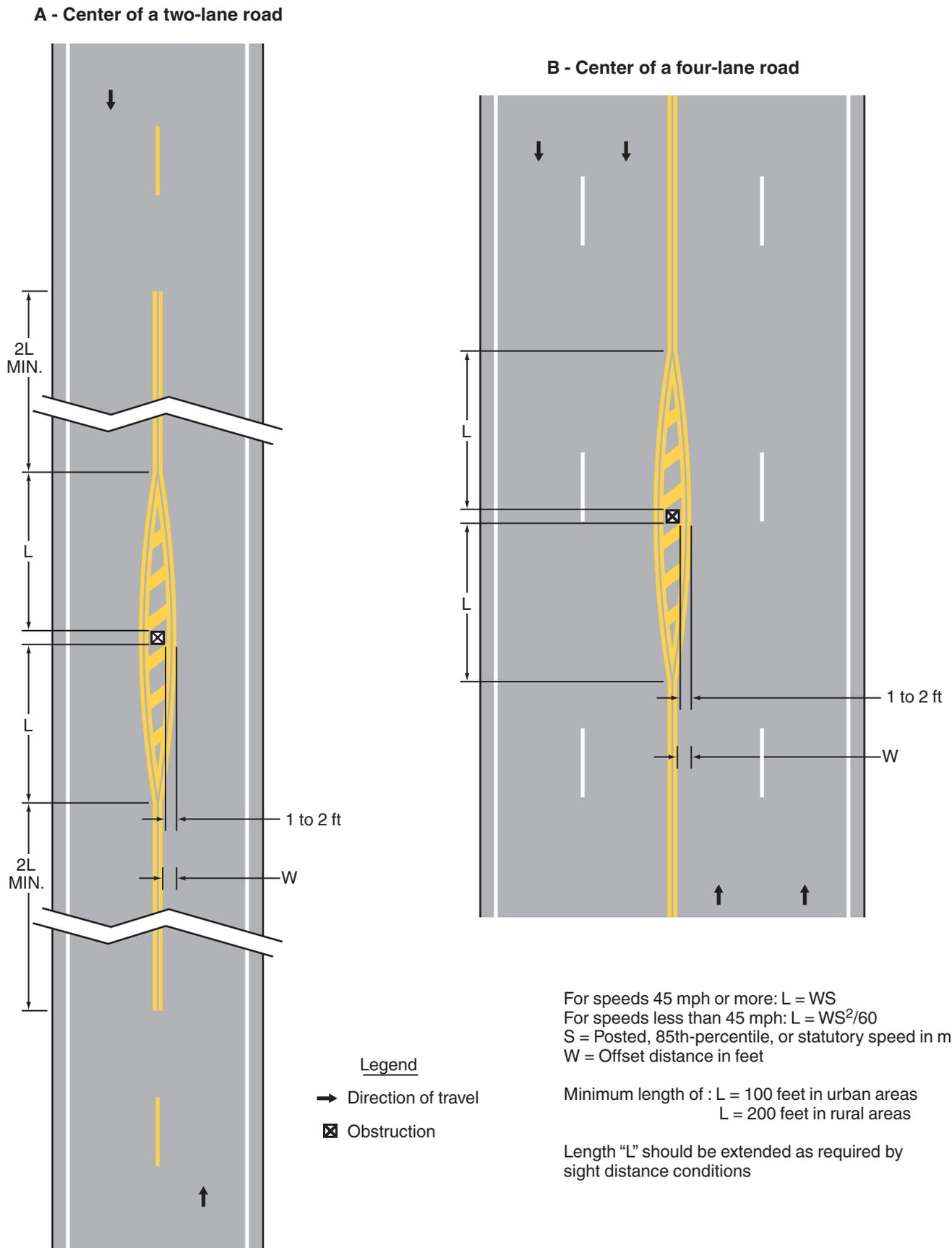
**Figure 3B-15. Examples of Applications of Markings for Obstructions in the Roadway**
