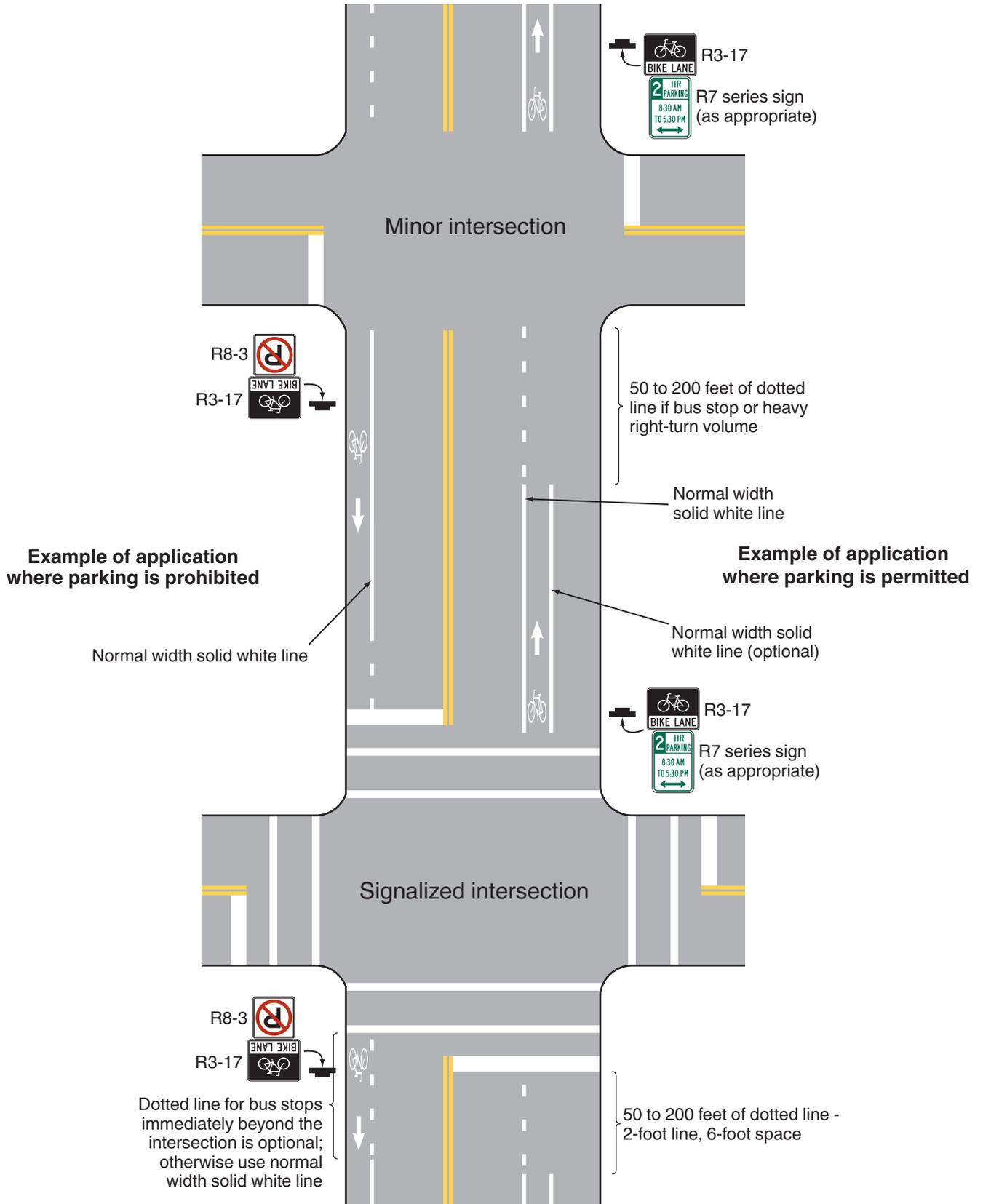
**Figure 9C-7. Bicycle Detector Pavement Marking**
