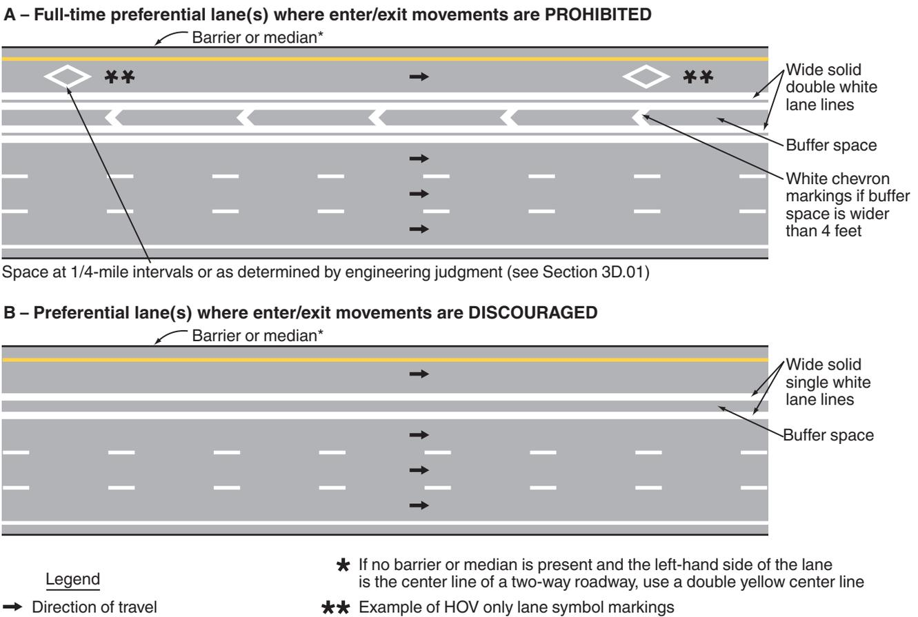
**Figure 3D-2. Markings for Buffer-Separated Preferential Lanes (Sheet 2 of 2)**
