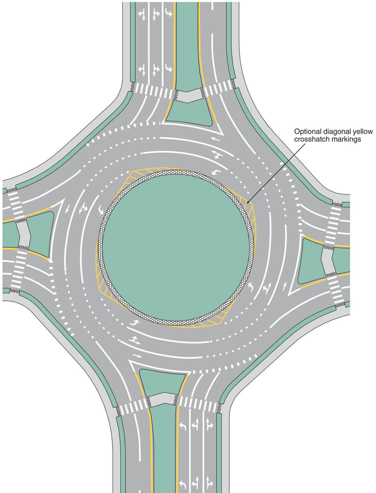
**Figure 3C-13. Example of Markings for Two Linked Roundabouts**
