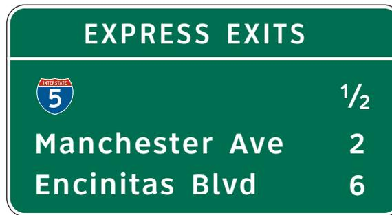
**Figure 2G-20. Example of a Comparative Travel Time Information Sign for Preferential or Managed Lanes**
