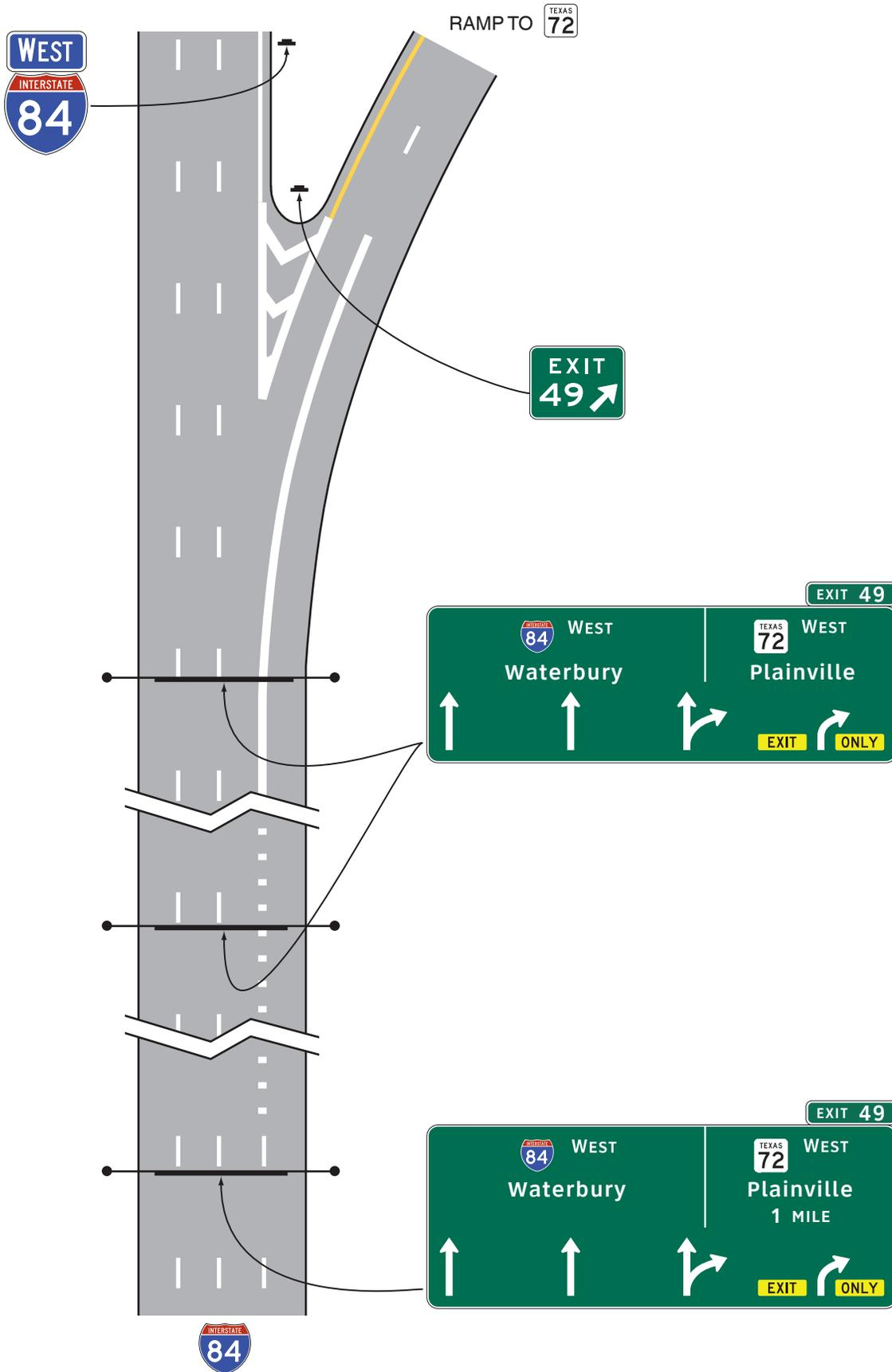
**Figure 2E-5. Overhead Arrow-per-Lane Guide Signs for a Two-Lane Exit to the Right with an Option Lane (Through Lanes Curve to the Left)**
