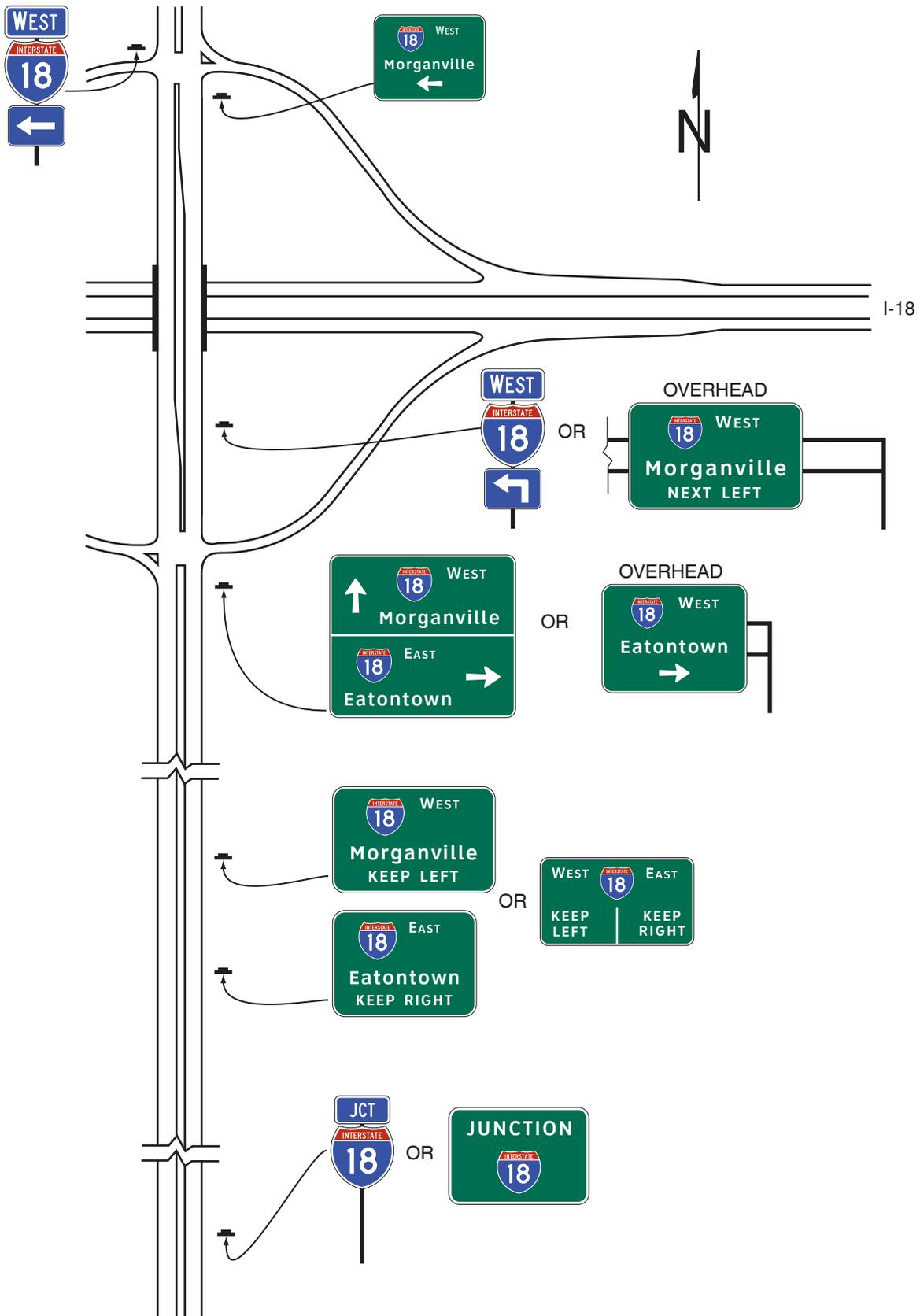
Figure 2D-14. Examples of Multi-Lane Crossroad Signing for a Partial Cloverleaf Interchange
