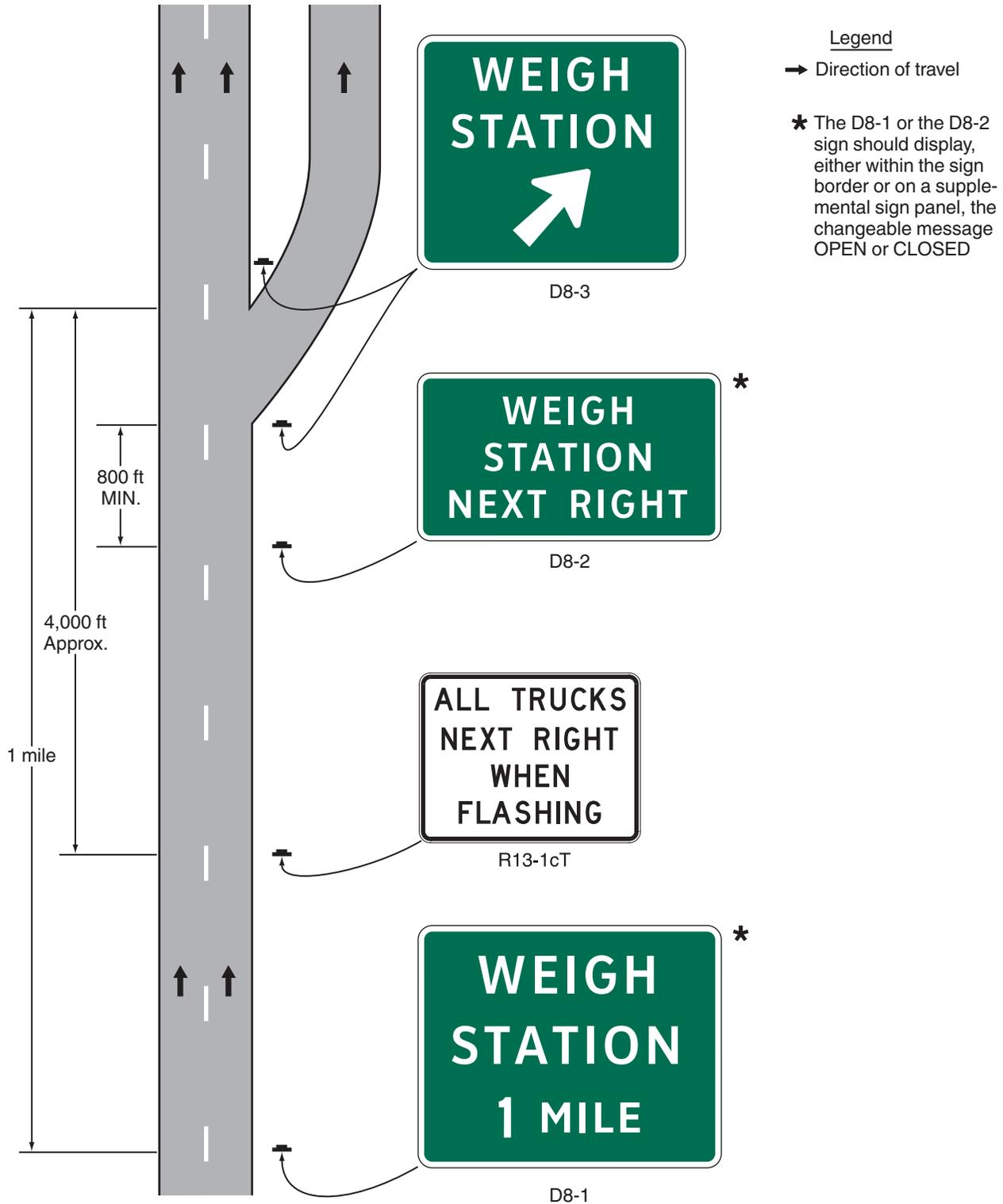
**Figure 2D-17TA. Commercial Motor Vehicle (CMV) Inspection Station Signing**
