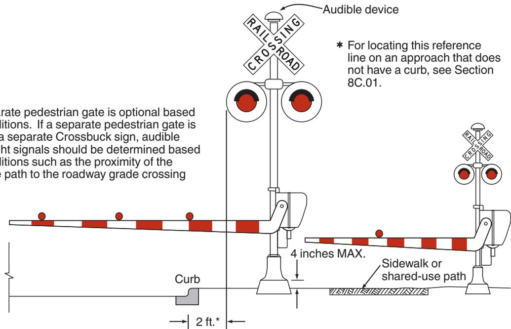
**Figure 8C-7. Examples of Placement of Pedestrian Gates**
