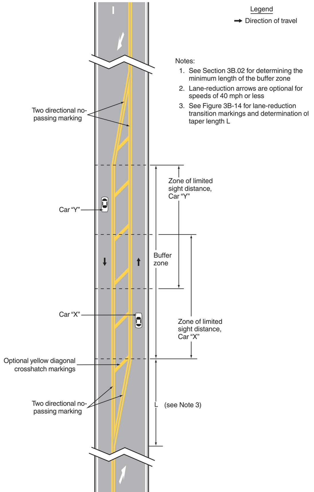
**Figure 3B-6. Example of Reversible Lane Marking Application**
